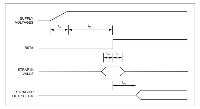
TABLE 7-5: POWER-UP/RESET TIMING PARAMETERS
