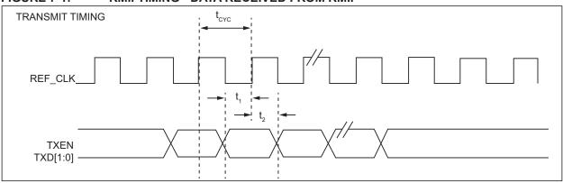
FIGURE 7-2: RMII TIMING - DATA INPUT TO RMII
