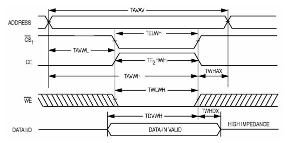
Note: The internal write time of the memory is defined by the overlap of  $\overline{\text{CS1}}$  Low and CE HIGH and  $\overline{\text{WE}}$  LOW. Both signals must be actived to initiate a write and either signal can terminate a write by going in actived. The data input setup and hold timing should be referenced to the actived edge of the signal that terminates the write. Data out is high impedance if  $\overline{\text{OE}} = V_{\text{IH}}$ .
