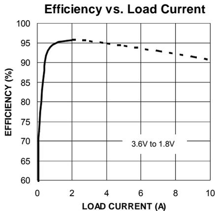
Figure 1. Efficiency Curve
