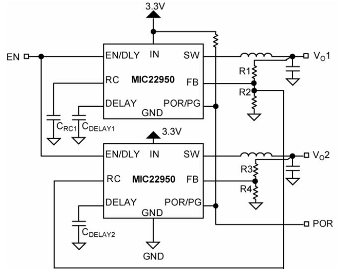
$C_{CR1} = 3.3nF, C_{RC2} = 0nF, C_{DELAY1} = C_{DELAY2} = 3.3nF$
