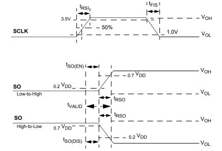
Figure 5. Valid Data Delay Time and Valid Time Waveforms
