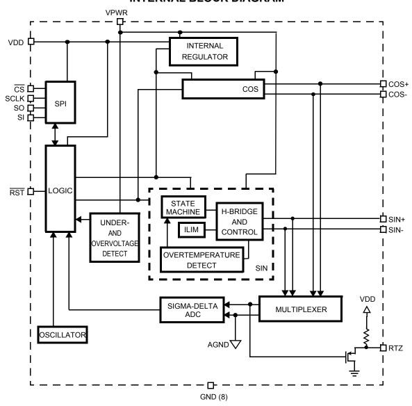
Figure 2. 33977 Simplified Internal Block Diagram
