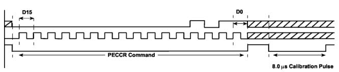
Figure 8. Gauge Enable and Clock Calibration Example
