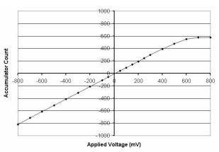
Figure 13. RTZ Accumulator (Typical)
