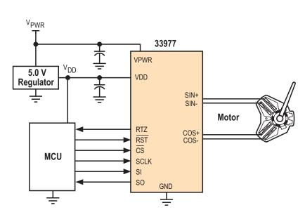
Figure 1. 33977 Simplified Application Diagram
