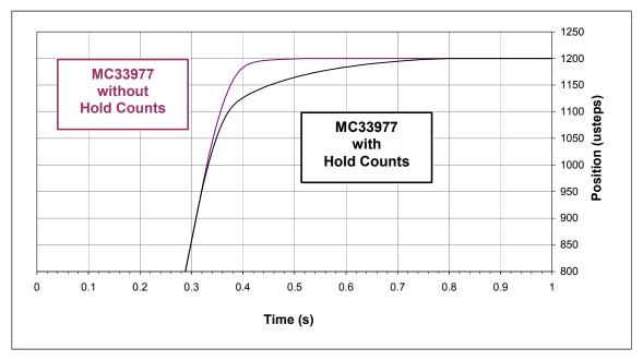
Figure 15. Deceleration Damping Response Examples
