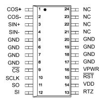
Figure 3. 33977 Pin Connections
