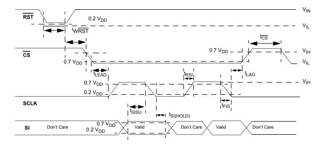
Figure 4. Input Timing Switching Characteristics
