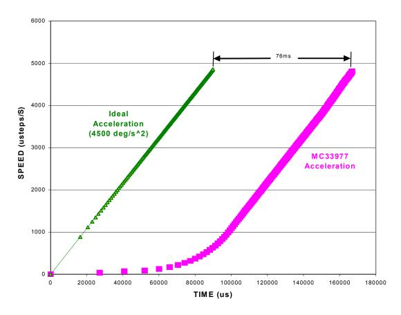
Figure 14. Acceleration Response Characteristics
