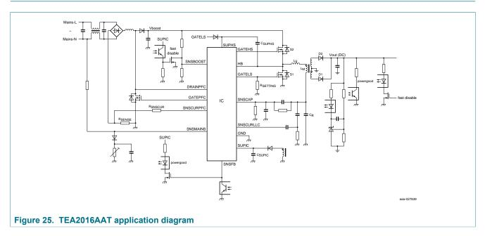
Digital controller for high-efficiency resonant power supply
