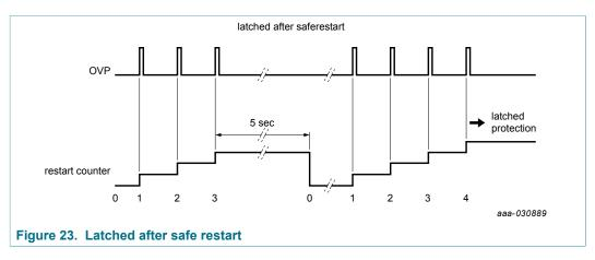
Figure 23 shows an example of when the OVP is set to latched after safe restart. Initially at an OVP, the system restarts. An internal counter is then set to '1'. If the protection is triggered again after the safe restart, the counter is increased. If the counter reaches the number as set with a parameter, the system latches. If the protection is not triggered within 5 seconds, the counter is reset.
