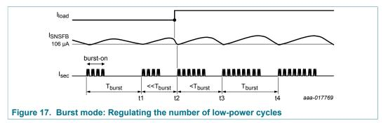
The system continuously measures the burst period from the start of the previous burston period to a new burst-on period. At t1, the measured burst period ( $t_{burst}$ ) equals the required  $T_{burst}$ . So, the next number of low-power cycles equals the number of previous low-power cycles. At a constant output power, the system expects that when the next burst-on period has the same number of low-power cycles as the previous burst-on period, the burst period ( $T_{burst}$ ) remains constant.
