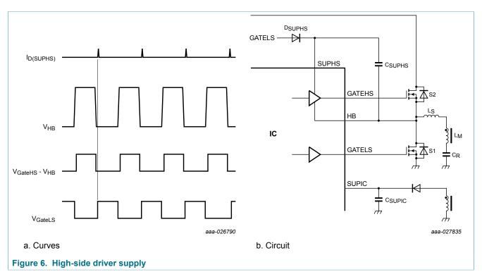
The external bootstrap buffer capacitor  $C_{SUPHS}$  supplies the high-side driver. The bootstrap capacitor is connected to the low-side driver supply, the GATELS pin, and the half-bridge node (HB) via an external diode (D<sub>SUPHS</sub>). When GATELS is active high and the HB node is pulled low,  $C_{SUPHS}$  is charged.
