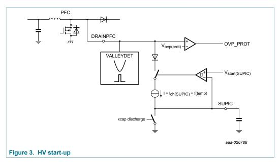
The maximum current of the internal current source is limited to  $I_{ch(SUPIC)}$ . To limit the IC dissipation, the charge current is reduced when the current source exceeds its maximum temperature ( $T_{SUPICcharger}$ ).
