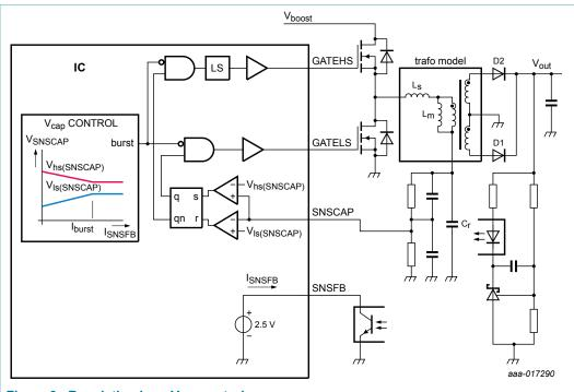
Figure 9. Regulation loop  $V_{cap}$  control
