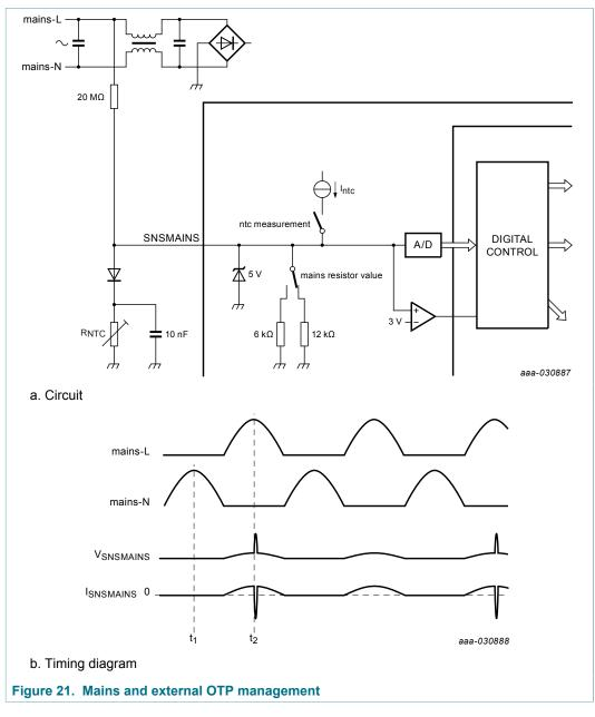
The TEA2016AAT continuously measures the SNSMAINS voltage via an A/D converter and waits until it detects a peak (t1). This peak value is internally stored and used as an input for the brownout/brownin detection and the mains compensation.
