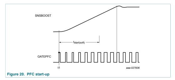
At t1, all conditions to start up the PFC are fulfilled. When the PFC starts switching, the maximum on-time is increased cycle-by-cycle from zero until the  $t_{on}$  regulation limits the on-time of the PFC external MOSFET.
