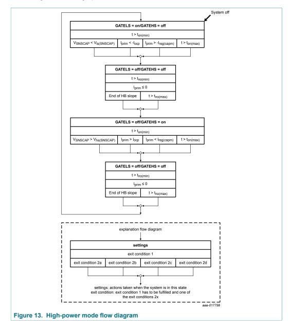
Initially, GATELS is on and GATEHS is off. The external bootstrap buffer capacitor  $(C_{SUPHS})$  is charged via the GATELS pin and an external diode. The system remains in this state for at least the minimum on-time  $(t_{on(min)})$  of GATELS. Before entering the next state, one of the following conditions must be fulfilled:
