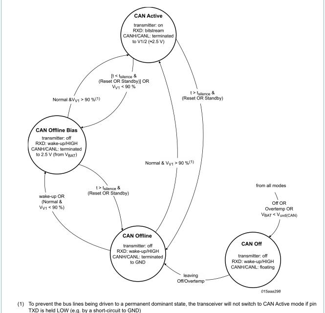
Fig 6. **CAN transceiver state machine**
