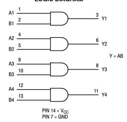
Pinout: 14-Lead Packages (Top View)
