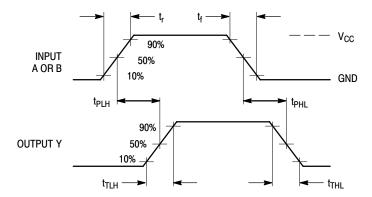
Figure 1. Switching Waveforms
