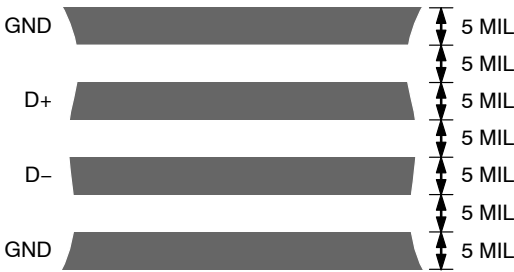
Figure 16. Typical Arrangement of Signal Tracks
