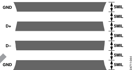
Figure 25. Arrangement of Signal Tracks
