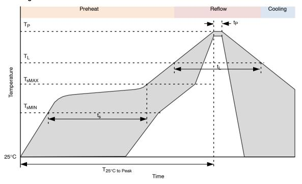
Figure 5. QFN40 Soldering Profile
