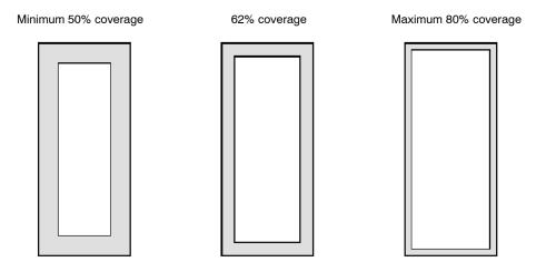
Figure 8. Solder Paste Application on Pins
