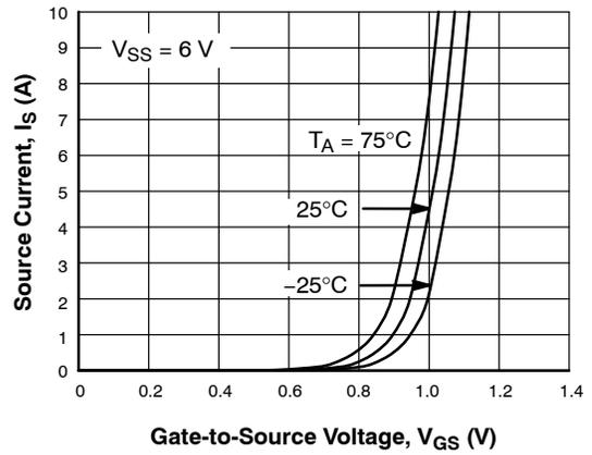
Figure 3. Transfer Characteristics
