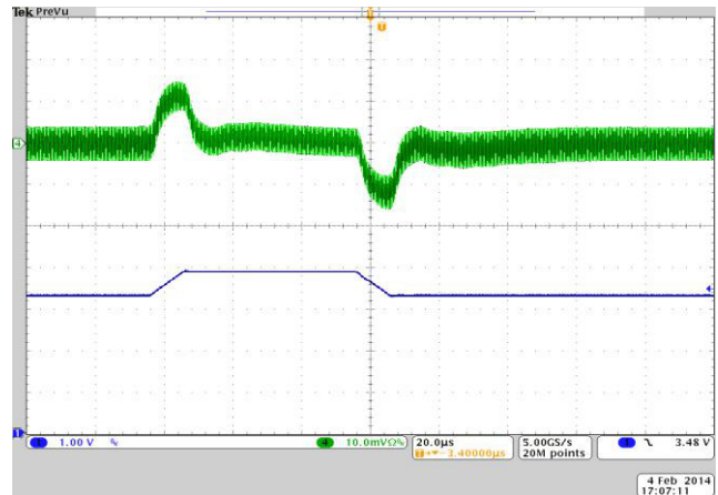
Figure 14. Line Transient, 200 mA Load, 10 µs Step
