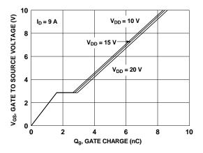
Figure 7. Gate Charge Characteristics
