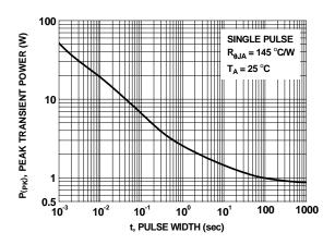
Figure 10. Single Pulse Maximum Power Dissipation
