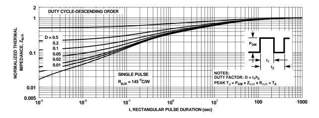
Figure 11. Junction-to-Ambient Transient Thermal Response Curve
