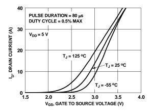
Figure 5. Transfer Characteristics
