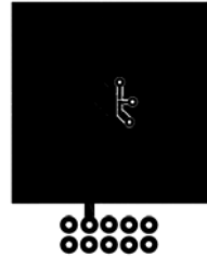
b. 55 °C/W when mounted on a 1 in 2 pad of 2 oz copper
