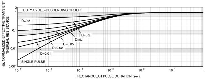
Figure 8. Junction-to-Case Transient Thermal Response
