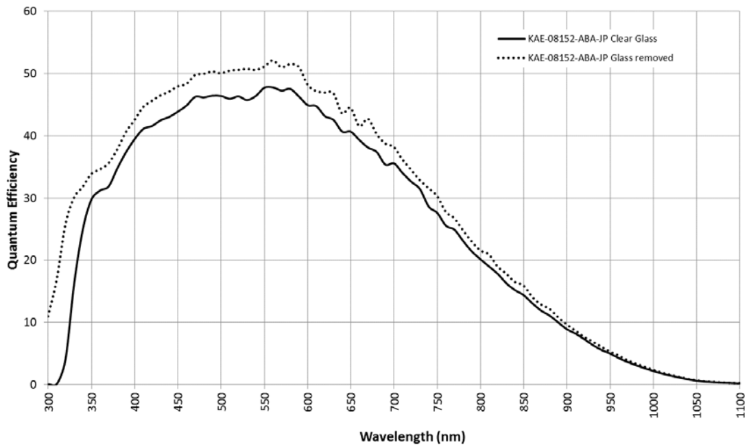
Figure 5. Quantum Efficiency of the KAE-08152-ABA-JP Configuration
