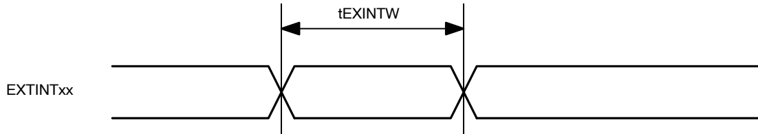
Figure 8. AC Characteristic – External Interrupt
