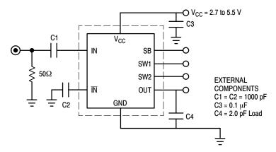
Figure 2. AC Test Circuit
