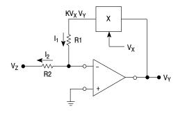
Figure 24. Basic Divide Circuit
