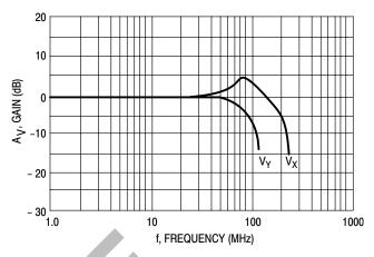
Figure 2. Transconductance Bandwidth
