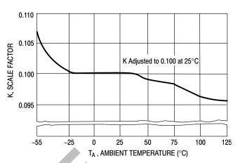
Figure 16. Scale Factor versus Temperature
