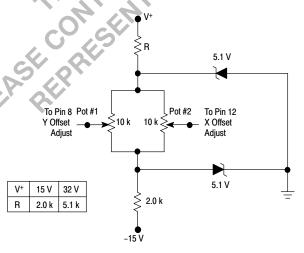
Figure 14. Offset Adjust Circuit (Alternate)
