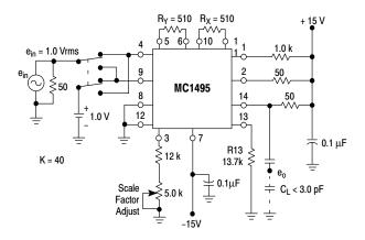
Figure 10. Bandwidth ( $R_L = 50 \Omega$ )
