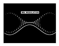
Figure 30. Amplitude Modulation
