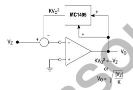
Figure 26. Basic Square Root Circuit
