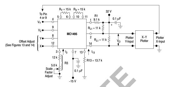
Figure 5. Linearity (Using X-Y Plotter Technique)
