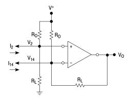
Figure 22. Level Shift Circuit
