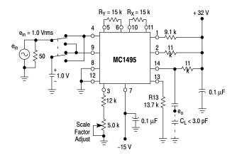
Figure 9. Bandwidth ( $R_L = 11 \text{ k}\Omega$ )
