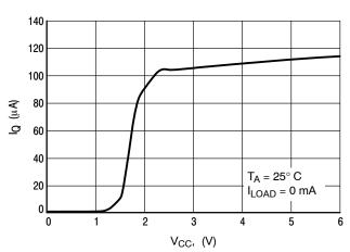
Figure 19. Quiescent Current versus Input Voltage
