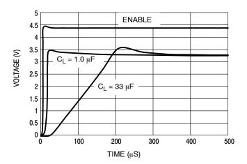
Figure 15. Enable Transient
