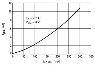
Figure 18. Ground Current versus Load Current
