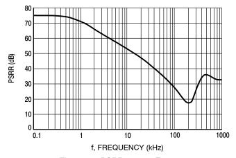
Figure 20. PSRR versus Frequency
