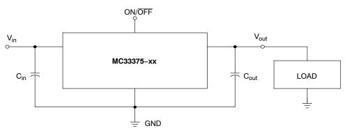
Figure 23. Typical Application Circuit
