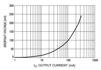
Figure 7. Dropout Voltage versus Output Current
