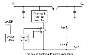
Figure 1. Simplified Block Diagram
