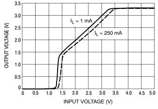
Figure 6. Output Voltage versus Input Voltage
