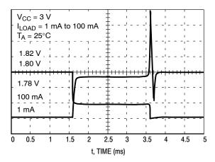
Figure 22. Load Transient Response
