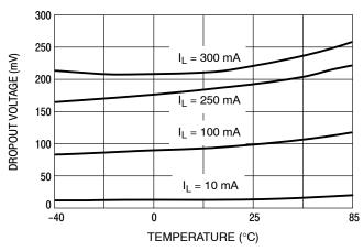
Figure 8. Dropout Voltage versus Temperature
