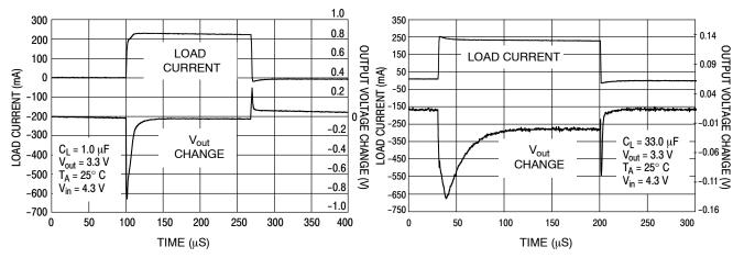
**Figure 4. Load Transient Response**
