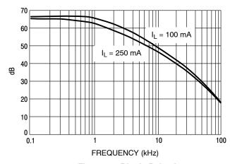
Figure 14. Ripple Rejection
