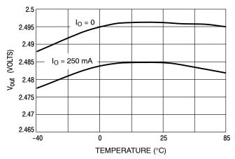
Figure 12. Output Voltage versus Ambient Temperature (V<sub>in</sub> = 12 V)
