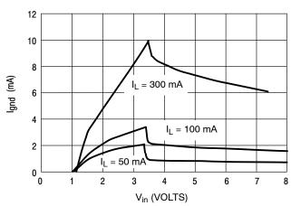
Figure 9. Ground Pin Current versus Input Voltage
