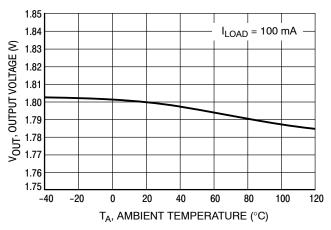
Figure 16. Output Voltage versus Temperature
