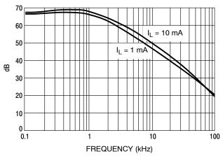
Figure 13. Ripple Rejection
