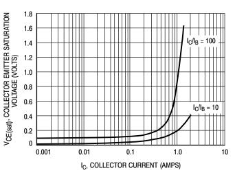
Figure 6. Collector Emitter Saturation Voltage versus Collector Current
