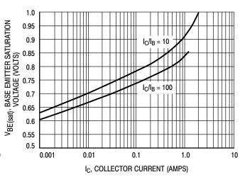
Figure 4. Base Emitter Saturation Voltage versus Collector Current
