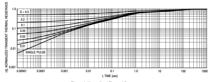
Figure 8. Normalized Thermal Response
