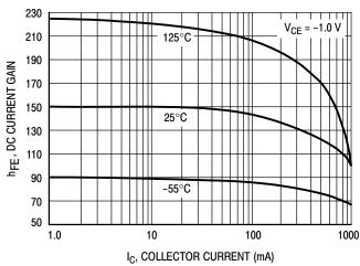
Figure 2. DC Current Gain versus Collector Current
