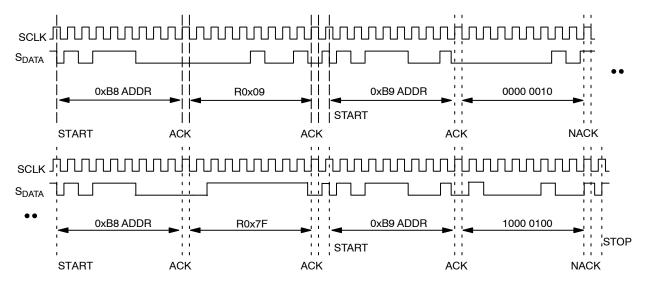
Figure 20. Timing Diagram Showing a Bytewise Read from R0x09; Returned Value 0x0284
