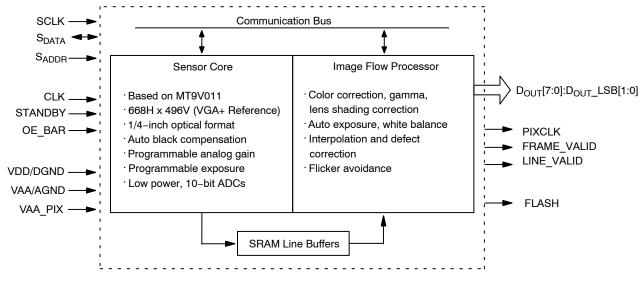
Figure 1. Chip Block Diagram
