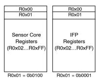
NOTE: Program R0x01 to select the desired space (0b0100 = sensor core registers, 0b0001 = IFP/SOC registers).
