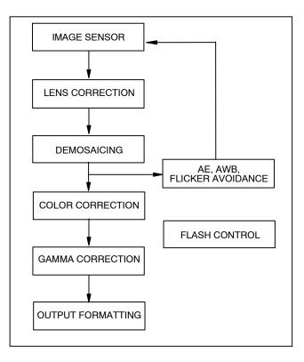
Figure 5. Image Flow Processor Block Diagram
