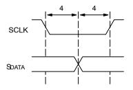
NOTE: SDATA is driven by an off-chip transmitter.
