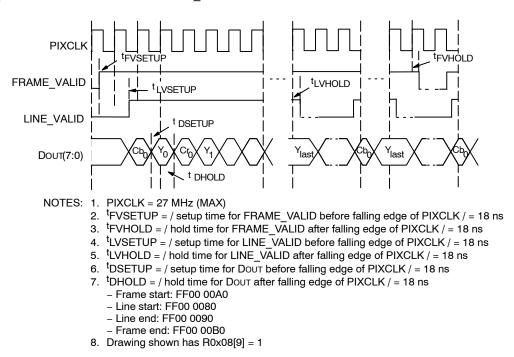
Figure 12. Data Output Timing Diagram
