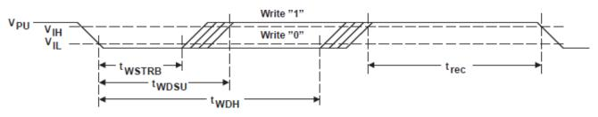
Figure 8. WRITE Bit Timing Diagram
