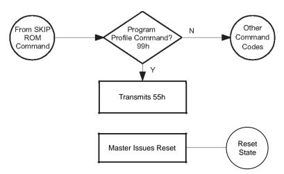
Figure 6. PROGRAM PROFILE Command Flow
