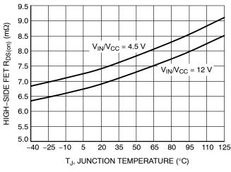
Figure 11. High-side R<sub>DS(on)</sub> vs. Temperature
