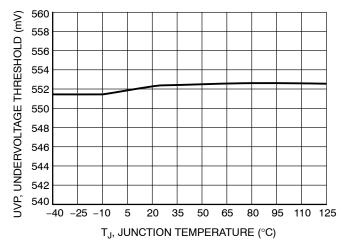
Figure 19. Output UVP vs. Junction Temperature
