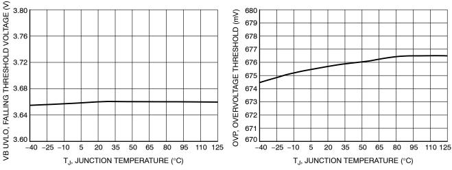
Figure 17. VB UVLO Falling Threshold vs. Junction Temperature
