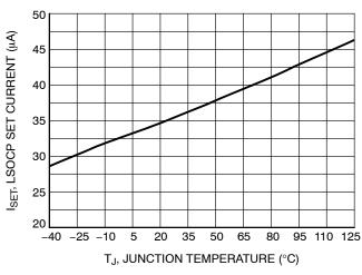
Figure 10. ISET Current vs. Temperature
