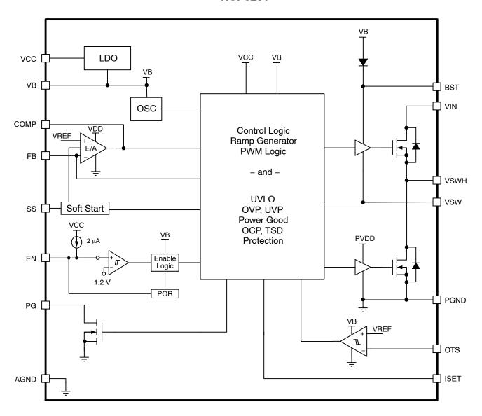
Figure 1. NCP3231 Block Diagram
