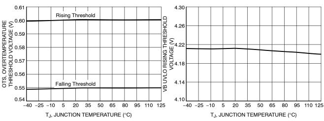
Figure 15. OTS Threshold vs. Temperature
