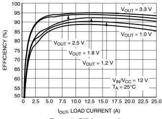
Figure 13. Efficiency vs. lout (Vin = 12 V)
