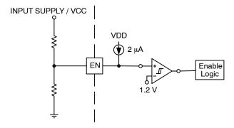
Figure 22. Enable Functional Block Diagram
