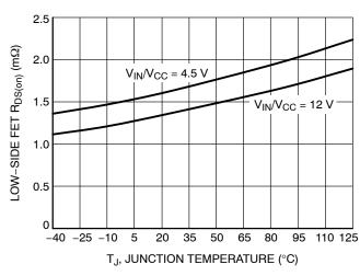
Figure 12. Low-side  $R_{DS(on)}$  vs. Temperature
