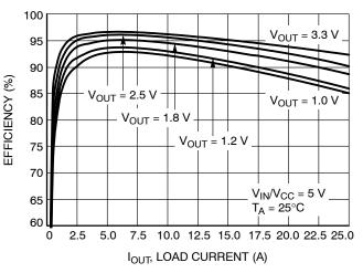
Figure 14. Efficiency vs. lout (Vin = 5 V)
