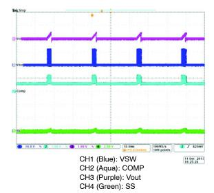
Figure 21. Typical Short Circuit Waveforms (Vin = 12 V)
