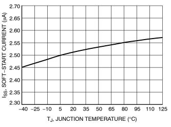
Figure 9. Soft-start Current vs. Temperature
