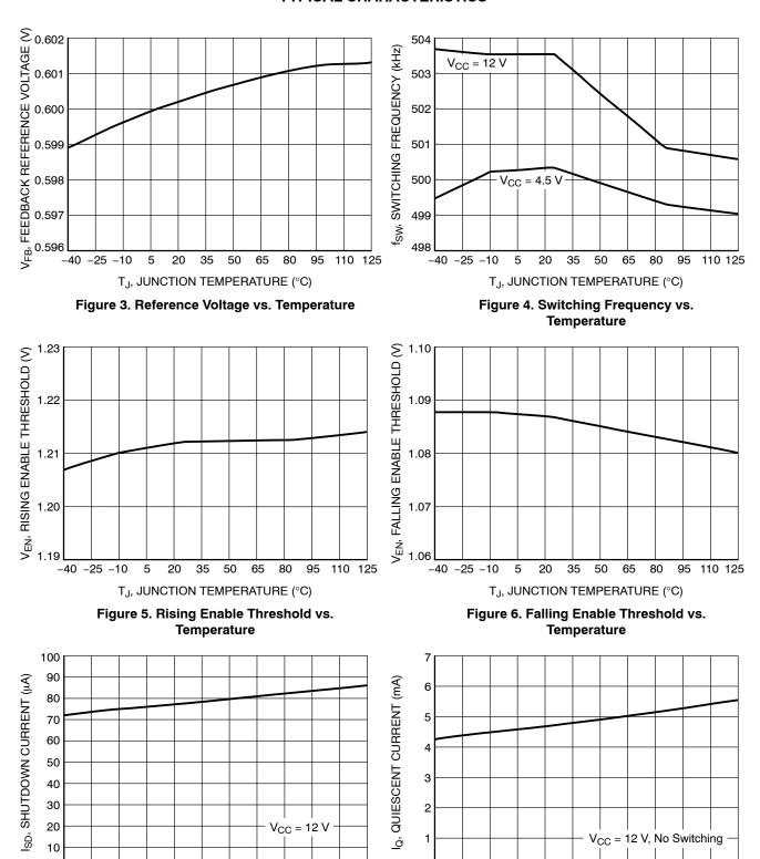
$T_{J},\,JUNCTION\,\,TEMPERATURE\,\,(^{\circ}C)$  Figure 7. Shutdown Current vs. Temperature
