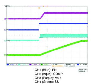
Figure 20. Typical Startup Waveforms (Vin = 12 V, lout = 25 A, Vout = 1 V)
