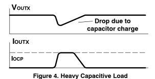
In case of overload, the current is limited to the I<sub>OCP</sub> value and the voltage value is reduced according to the load by the following relation:
