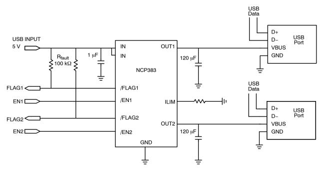
Figure 1. Typical Application Circuit: NCP383xMUAJxx
