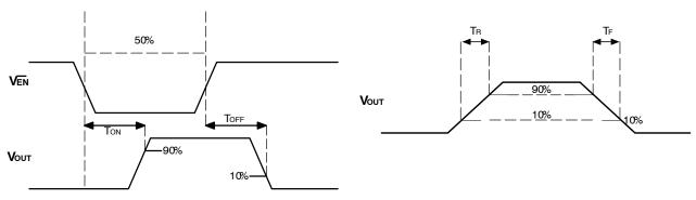
Figure 3. Ton, Toff, Trise, and Tfall
