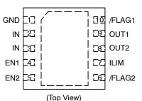
Exposed pad must be soldered to PCB Ground plane.
