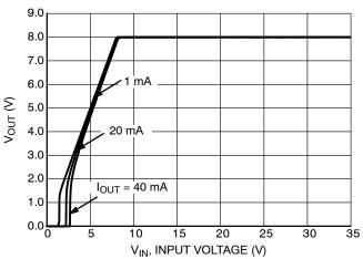
Figure 16. Output Voltage vs. Input Voltage, 8.0 V Version
