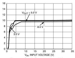
Figure 12. Supply Current vs. Input Voltage
