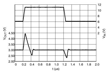
Figure 23. Line Transients, 3.0 V Version,  $t_R = t_F = 5~\mu s,~l_{OUT} = 1~mA$
