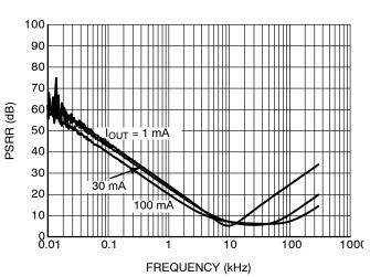
Figure 18. PSRR, 5.0 V Version,  $V_{IN}$  = 8.0 V
