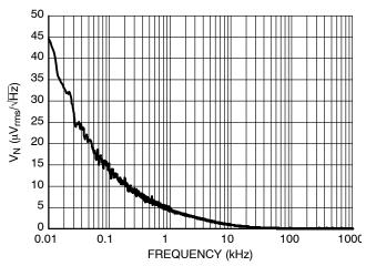
Figure 22. Output Voltage Noise, 8.0 V version,  $V_{IN}$  = 11.0 V,  $I_{OUT}$  = 30 mA
