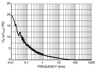
Figure 21. Output Voltage Noise, 5.0 V Version,  $V_{IN} = 8.0 \text{ V}, I_{OUT} = 30 \text{ mA}$
