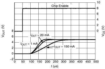
Figure 30. Start-up, 5.0 V Version,  $V_{IN}$  = 8.0 V
