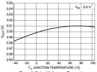
Figure 9. Output Voltage vs. Temperature, 3.0 V Version
