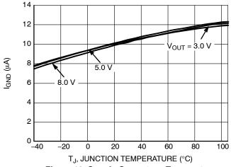
Figure 13. Supply Current vs. Temperature
