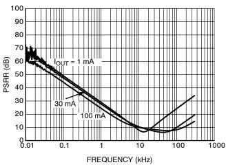
Figure 17. PSRR, 3.0 V Version,  $V_{IN}$  = 6.0 V
