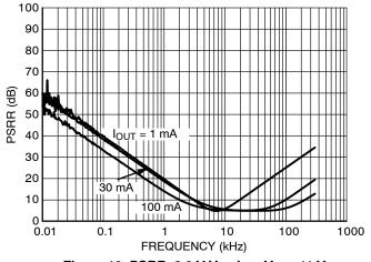
Figure 19. PSRR, 8.0 V Version,  $V_{IN}$  = 11 V
