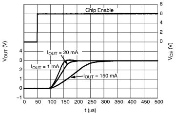
Figure 29. Start-up, 3.0 V Version, V<sub>IN</sub> = 6.0 V
