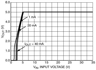
Figure 15. Output Voltage vs. Input Voltage, 5.0 V Version
