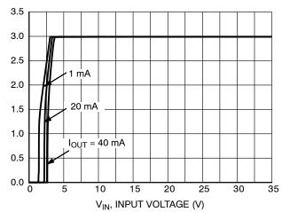
Figure 14. Output Voltage vs. Input Voltage, 3.0 V Version
