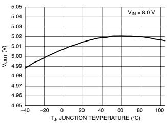
Figure 10. Output Voltage vs. Temperature, 5.0 V Version
