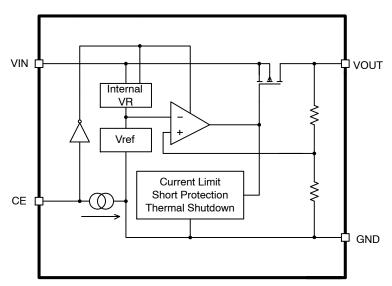
Figure 2. Simplified Schematic Block Diagram
