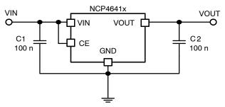
Figure 32. Typical Application Schematic
