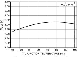
Figure 11. Output Voltage vs. Temperature, 8.0 V Version
