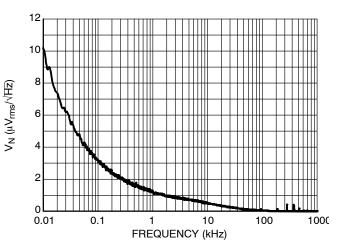
Figure 20. Output Voltage Noise, 3.0 V Version,  $V_{IN} = 6.0 \text{ V}, I_{OUT} = 30 \text{ mA}$
