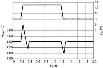
Figure 24. Line Transients, 5.0 V Version,  $t_R = t_F = 5~\mu s,~l_{OUT} = 1~mA$
