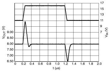
Figure 25. Line Transients, 8.0 V Version,  $t_R = t_F = 5~\mu s, \, l_{OUT} = 1~mA$
