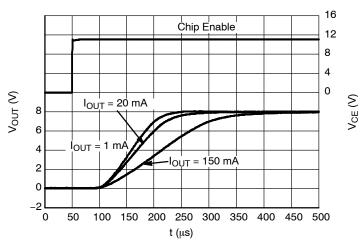
Figure 31. Start-up, 8.0 V Version, V<sub>IN</sub> = 11.0 V
