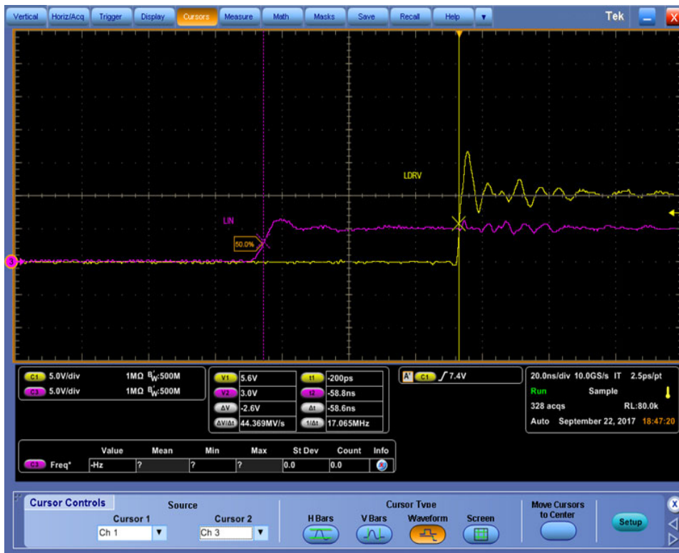
Figure 30. Low Side Turn-ON Propagation Delay (NCP51530A)
