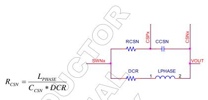
The individual phase current is summed into to the PWM comparator feedback in this way current is balanced is via a current mode control approach.
