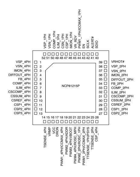
Figure 2. Pinout Diagram
