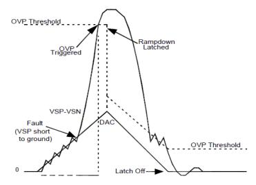
Figure 16. OVP Behavior at Startup
