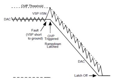
Figure 15. OVP During Normal Operation Mode
