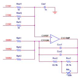
The DC gain equation for the current sensing:
