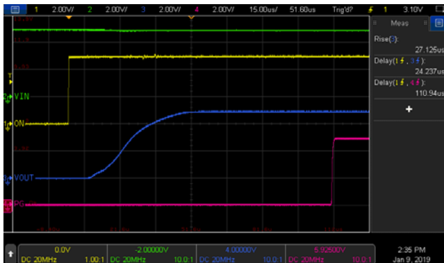
Figure 29. Rise Time vs. Input Voltage
