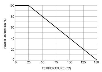
Figure 2. Steady State Power Derating
