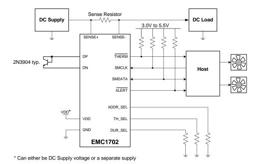
Figure 4.1 EMC1702 System Diagram
