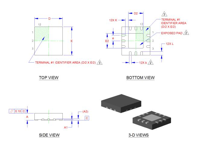
Figure 6.1 12-Pin QFN 4mm x 4mm Package Drawings
