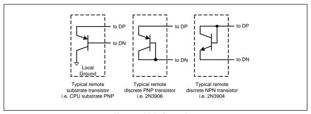
**Figure 4.3 Diode Connections**
