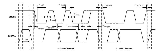
Figure 3.1 SMBus Timing Diagram
