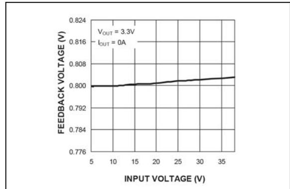
**FIGURE 2-5:** Feedback Voltage vs. Input Voltage (MIC2101).
