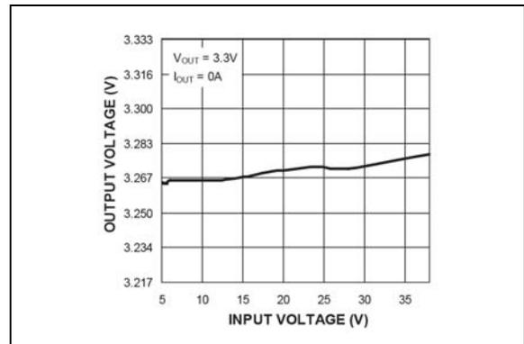
**FIGURE 2-6:** Output Voltage vs. Input Voltage (MIC2101).
