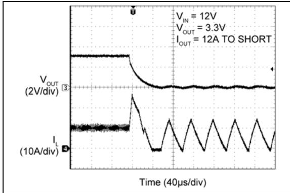
**FIGURE 2-67:** Short-Circuit.
