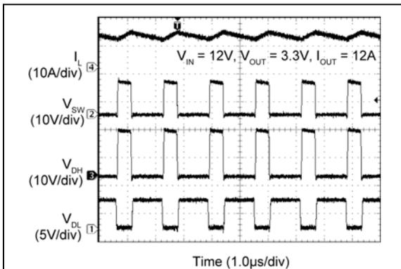
**FIGURE 2-75:** MIC2101 Switching Waveforms ( $I_{OUT} = 12A$ ).
