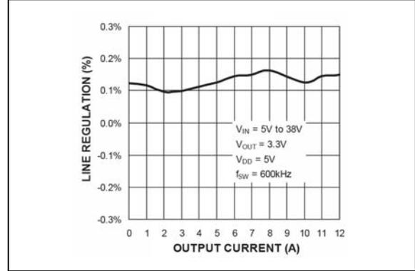
**FIGURE 2-30:** Line Regulation vs. Output Current (MIC2102).
