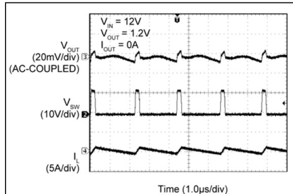
**FIGURE 2-84:** MIC2102 Switching Waveforms ( $I_{OUT} = 0A$ ).
