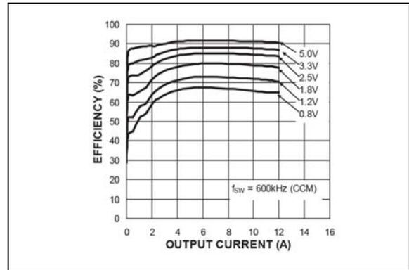
**FIGURE 2-16:** Efficiency ( $V_{IN} = 18V$ ) vs. Output Current (MIC2101).
