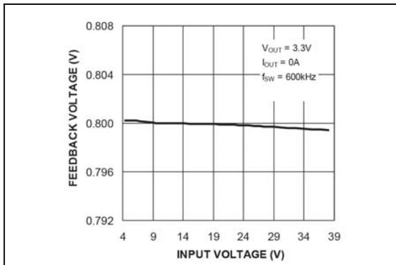
**FIGURE 2-20:** Feedback Voltage vs. Input Voltage (MIC2102).
