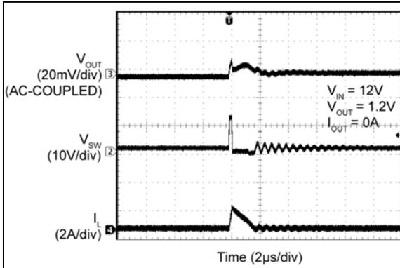
**FIGURE 2-85:** MIC2101 Switching Waveforms ( $I_{OUT} = 0A$ ).
