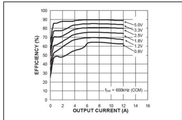
**FIGURE 2-17:** Efficiency ( $V_{IN} = 24V$ ) vs. Output Current (MIC2101).
