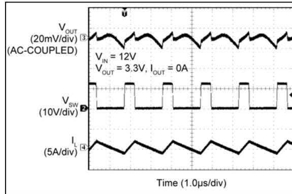
**FIGURE 2-72:** MIC2102 Switching Waveforms ( $I_{OUT} = 0A$ ).
