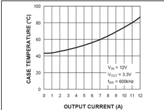
**FIGURE 2-37:** Case Temperature\* ( $V_{IN} = 12V$ ) vs. Output Current.
