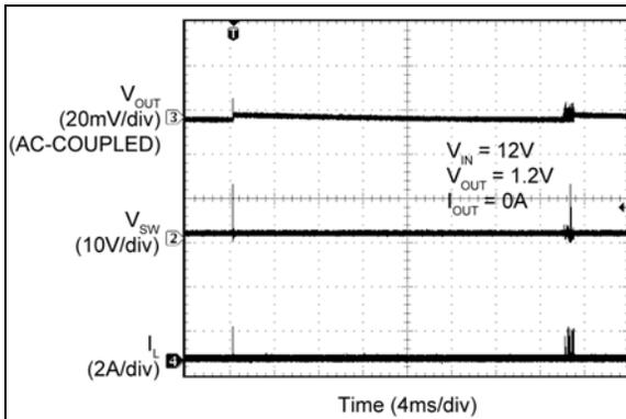
**FIGURE 2-86:** MIC2101 Switching Waveforms ( $I_{OUT} = 0A$ ).
