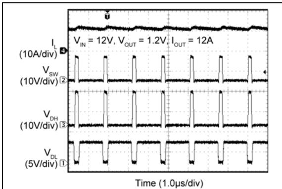
**FIGURE 2-87:** MIC2101 Switching Waveforms ( $I_{OUT} = 12A$ ).
