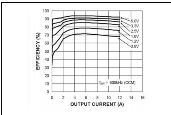
**FIGURE 2-15:** Efficiency ( $V_{IN} = 12V$ ) vs. Output Current (MIC2101).
