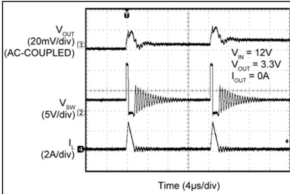
**FIGURE 2-73:** MIC2101 Switching Waveforms ( $I_{OUT} = 0A$ ).
