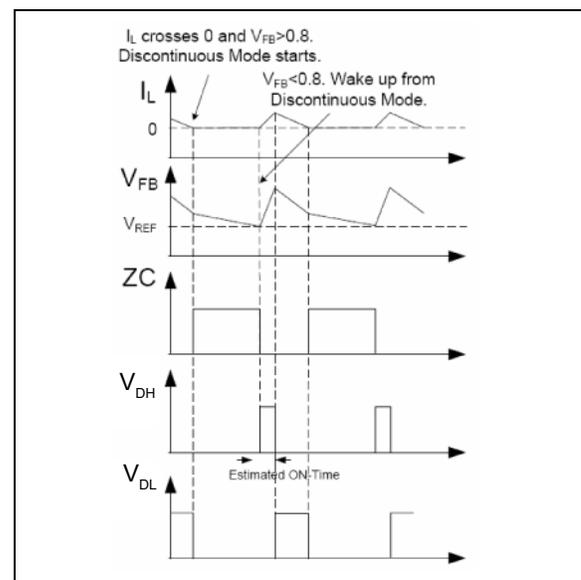
**FIGURE 4-3:** MIC2101 Control Loop Timing (Discontinuous Mode).
