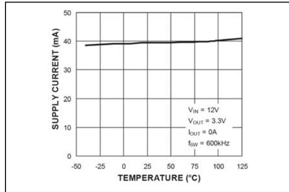
**FIGURE 2-24:**  $V_{IN}$  Operating Supply Current vs. Temperature (MIC2102).
