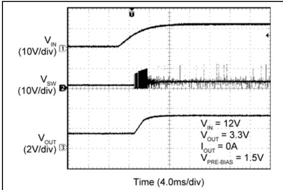
**FIGURE 2-61:** MIC2101  $V_{IN}$  Start-Up with Pre-Biased Output.
