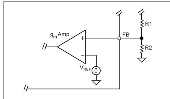
**FIGURE 5-3:** Voltage-Divider Configuration.
