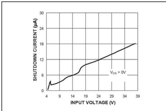
**FIGURE 2-44:**  $V_{IN}$  Shutdown Current vs. Input Voltage.
