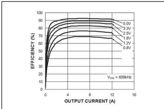
**FIGURE 2-33:** Efficiency ( $V_{IN} = 18V$ ) vs. Output Current (MIC2102).
