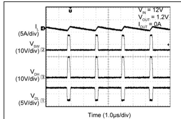
**FIGURE 2-90:** MIC2102 Switching Waveforms ( $I_{OUT} = 0A$ ).
