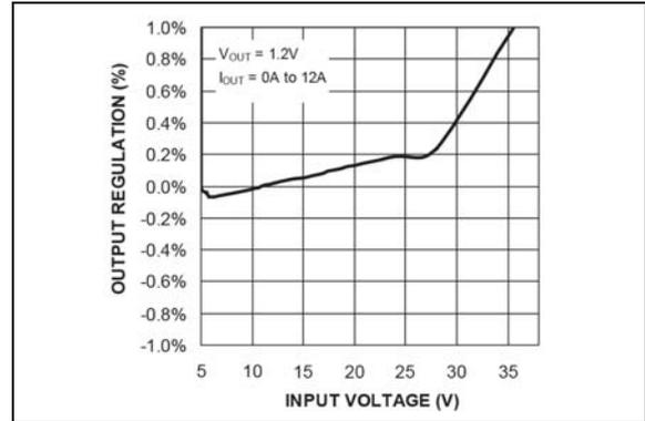
**FIGURE 2-4:** Output Regulation vs. Input Voltage (MIC2101).
