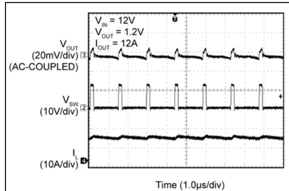
**FIGURE 2-83:** MIC2102 Switching Waveforms ( $I_{OUT} = 12A$ ).
