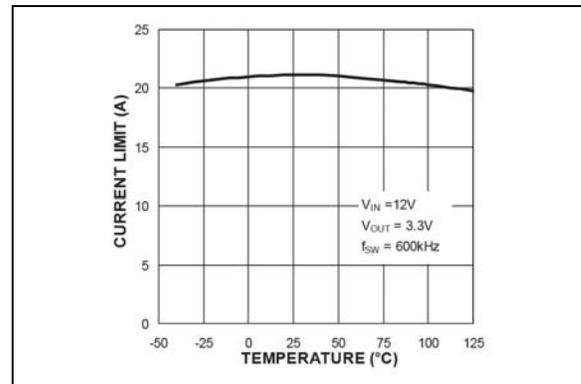
**FIGURE 2-53:** Output Peak Current Limit vs. Temperature.
