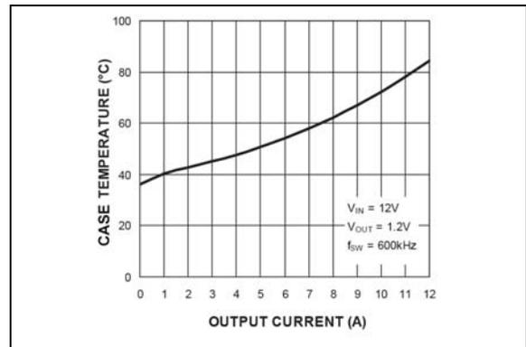
**FIGURE 2-41:** Case Temperature\* ( $V_{IN} = 12V$ ) vs. Output Current.
