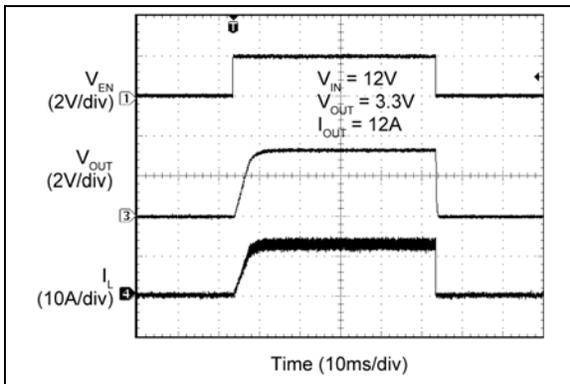
**FIGURE 2-62:** Enable Turn-On/Turn-Off.
