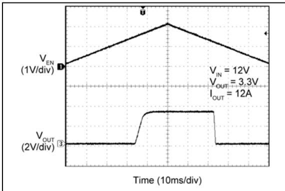
**FIGURE 2-63:** Enable Thresholds.
