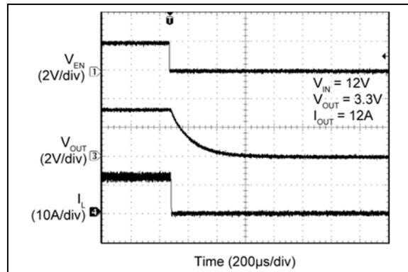
**FIGURE 2-59:** Enable Turn-Off Delay and Fall Time.
