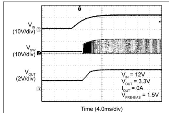
**FIGURE 2-60:** MIC2102  $V_{IN}$  Start-Up with Pre-Biased Output.
