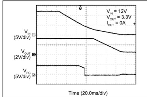
**FIGURE 2-82:** Power Good at  $V_{IN}$  Soft Turn-Off.
