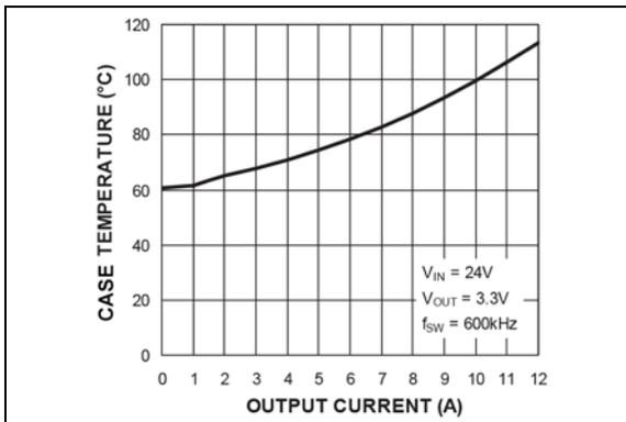
**FIGURE 2-38:** Case Temperature\* ( $V_{IN} = 24V$ ) vs. Output Current.
