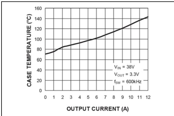
**FIGURE 2-39:** Case Temperature\* ( $V_{IN} = 38V$ ) vs. Output Current.
