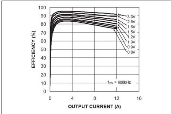
**FIGURE 2-31:** Efficiency ( $V_{IN} = 5V$ ) vs. Output Current (MIC2102).
