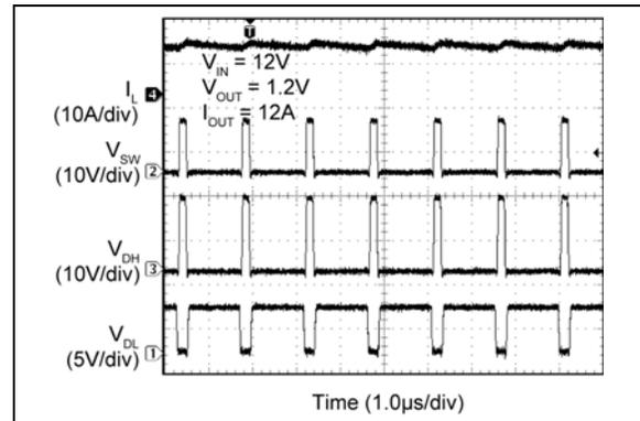
**FIGURE 2-89:** MIC2102 Switching Waveforms ( $I_{OUT} = 12A$ ).
