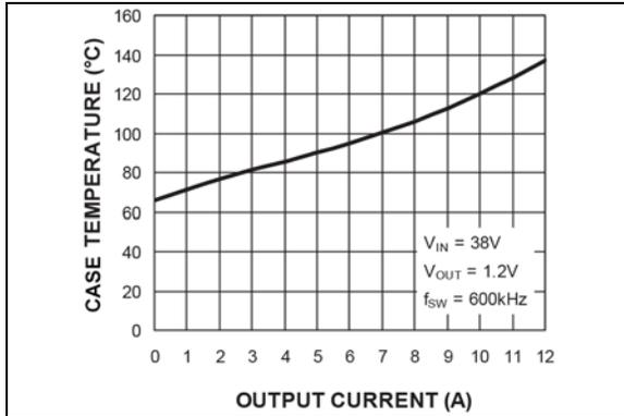
**FIGURE 2-43:** Case Temperature\* ( $V_{IN} = 38V$ ) vs. Output Current.
