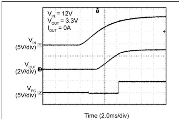
**FIGURE 2-81:** Power Good at  $V_{IN}$  Soft Turn-On.
