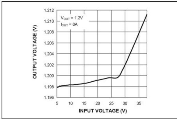
**FIGURE 2-7:** Output Voltage vs. Input Voltage (MIC2101).
