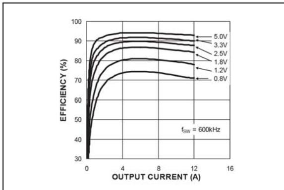
**FIGURE 2-32:** Efficiency ( $V_{IN} = 12V$ ) vs. Output Current (MIC2102).
