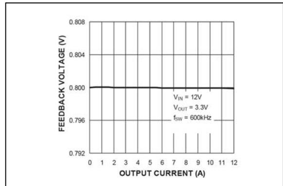
**FIGURE 2-29:** Feedback Voltage vs. Output Current (MIC2102).
