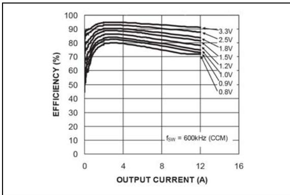
**FIGURE 2-14:** Efficiency ( $V_{IN} = 5V$ ) vs. Output Current (MIC2101).
