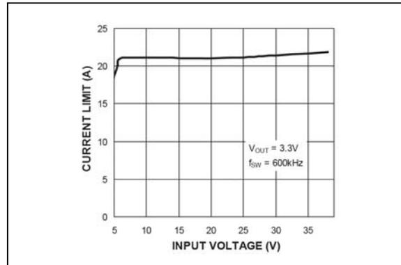
**FIGURE 2-48:** Output peak Current Limit vs. Input Voltage.
