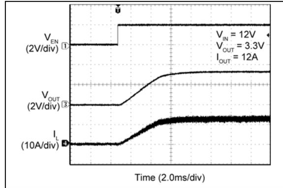
**FIGURE 2-58:** Enable Turn-On Delay and Rise Time.
