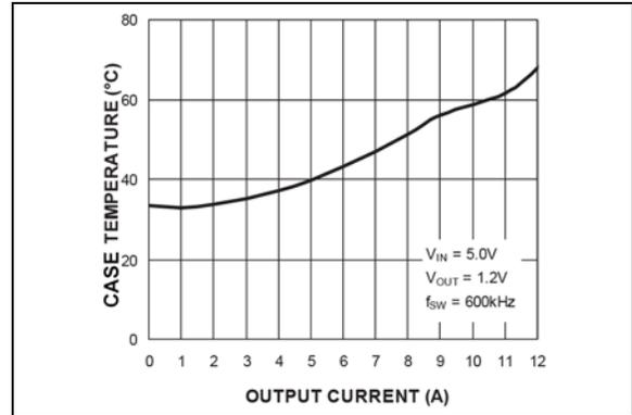
**FIGURE 2-40:** Case Temperature\* ( $V_{IN} = 5.0V$ ) vs. Output Current.
