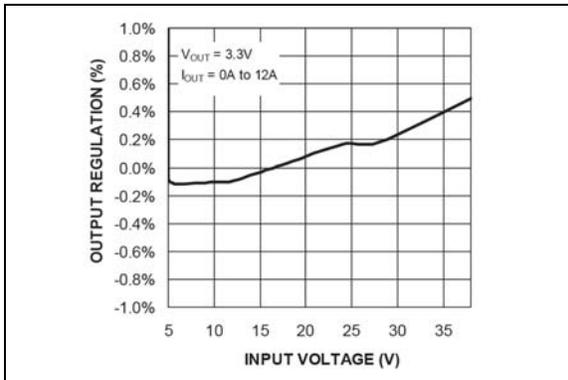
**FIGURE 2-2:** Output Regulation vs. Input Voltage (MIC2101).
