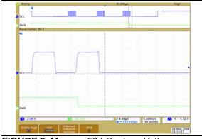
**FIGURE 2-41:** 50 k $\Omega$  – Low-Voltage Decrement Wiper Settling Time (V<sub>DD</sub> = 2.7V) (1  $\mu$ s/Div).
