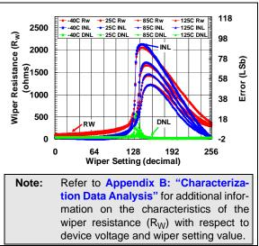
**FIGURE 2-11:** 5 kΩ Rheo Mode –  $R_W(Ω)$ , INL (LSb), DNL (LSb) vs. Wiper Setting and Ambient Temperature ( $V_{DD} = 1.8V$ ).
