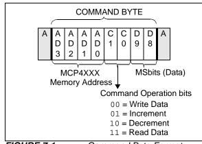
FIGURE 7-1: Command Byte Format.
