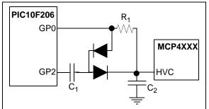
FIGURE 8-2:MCP4XXX NonvolatileDigital Potentiometer Evaluation Board(MCP402XEV) Implementation to Generate theV<sub>IHH</sub> Voltage.
