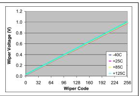
**FIGURE B-8:** Wiper Voltage  $(V_W)$  vs. Wiper Code  $(V_{DD} = 3.0V, I_W = 190 \ \mu A)$ .
