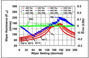
**FIGURE 2-33:** 50 k $\Omega$  Pot Mode –  $R_W(\Omega)$ , INL (LSb), DNL (LSb) vs. Wiper Setting and Ambient Temperature (V<sub>DD</sub> = 3.0V).
