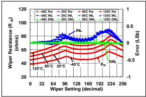
**FIGURE 2-22:** 10 k $\Omega$  Rheo Mode –  $R_W(\Omega)$ , INL (LSb), DNL (LSb) vs. Wiper Setting and Ambient Temperature (V<sub>DD</sub> = 5.5V).
