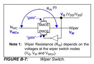
So, looking at the wiper voltage (V<sub>W</sub>) for the 3.0V and 1.8V data gives the graphs in Figure B-8 and Figure B-9. In the 1.8V graph, as the V<sub>W</sub> approaches 0.8V, the voltage increases nonlinearly. Since V = I \* R, and the current (I<sub>W</sub>) is constant, it means that the device resistance increased nonlinearly at around wiper code 160.
