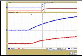
**FIGURE 2-42:** 50  $k\Omega$  – Power-Up Wiper Response Time (1  $\mu$ s/Div).
