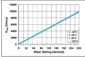
**FIGURE 2-26:** 10 k $\Omega$  – R<sub>WB</sub> ( $\Omega$ ) vs. Wiper Setting and Ambient Temperature.
