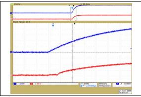
**FIGURE 2-29:** 10 k $\Omega$  – Power-Up Wiper Response Time (1  $\mu$ s/Div).
