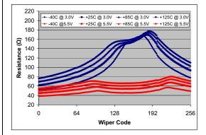
**FIGURE B-3:** Wiper Resistance ( $R_W$ ) vs. Wiper Code and Temperature ( $V_{DD} = 5.5V$ ,  $I_W = 900$  UA;  $V_{DD} = 3.0V$ ,  $I_W = 480 \mu A$ ).
