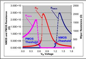
**FIGURE B-11:** NMOS and PMOS Transistor Resistance ( $R_{NMOS}$ ,  $R_{PMOS}$ ) and Wiper Resistance ( $R_W$ ) VS.  $V_{IN}$ ( $V_{DD} = 3.0V$ ).
