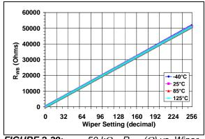
**FIGURE 2-39:** 50 k $\Omega$  – R<sub>WB</sub> ( $\Omega$ ) vs. Wiper Setting and Ambient Temperature.
