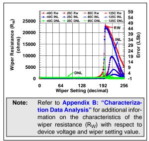
**FIGURE 2-50:** 100 k $\Omega$  Rheo Mode –  $R_W$  ( $\Omega$ ), INL (LSb), DNL (LSb) vs. Wiper Setting and Ambient Temperature ( $V_{DD} = 1.8V$ ).
