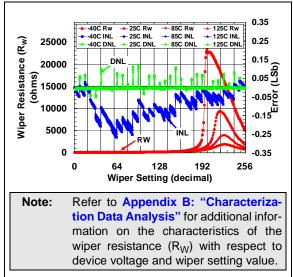
**FIGURE 2-47:** 100 k $\Omega$  Pot Mode –  $R_W(\Omega)$ , INL (LSb), DNL (LSb) vs. Wiper Setting and Ambient Temperature (V<sub>DD</sub> = 1.8V).
