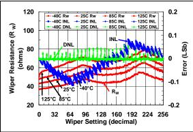
**FIGURE 2-45:** 100 k $\Omega$  Pot Mode –  $R_W(\Omega)$ , INL (LSb), DNL (LSb) vs. Wiper Setting and Ambient Temperature (V<sub>DD</sub> = 5.5V).
