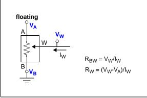
FIGURE 2-66: R<sub>BW</sub> and R<sub>W</sub> Measurement.
