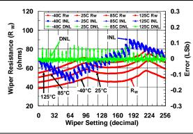
**FIGURE 2-6:**  $5 \ k\Omega \ \text{Pot} \ \text{Mode} - R_W(\Omega)$ , INL (LSb), DNL (LSb) vs. Wiper Setting and Ambient Temperature (V<sub>DD</sub> = 5.5V).
