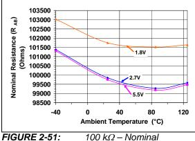
Resistance ( $\Omega$ ) vs. Ambient Temperature and  $V_{DD}$ .
