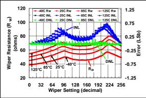
**FIGURE 2-9:** 5 k $\Omega$  Rheo Mode –  $R_W(\Omega)$ , INL (LSb), DNL (LSb) vs. Wiper Setting and Ambient Temperature (V<sub>DD</sub> = 5.5V).
