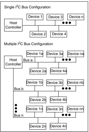
**FIGURE 8-5:** Typical Application  $l^2C$  Bus Configurations.
