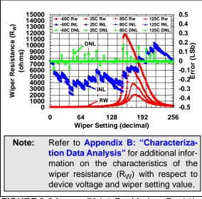
**FIGURE 2-34:** 50 k $\Omega$  Pot Mode –  $R_W(\Omega)$ , INL (LSb), DNL (LSb) vs. Wiper Setting and Ambient Temperature ( $V_{DD} = 1.8V$ ).
