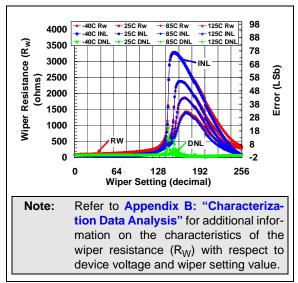
**FIGURE 2-24:** 10 k $\Omega$  Rheo Mode –  $R_W(\Omega)$ , INL (LSb), DNL (LSb) vs. Wiper Setting and Ambient Temperature ( $V_{DD} = 1.8V$ ).
