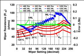
**FIGURE 2-35:** 50 k $\Omega$  Rheo Mode –  $R_W(\Omega)$ , INL (LSb), DNL (LSb) vs. Wiper Setting and Ambient Temperature (V<sub>DD</sub> = 5.5V).
