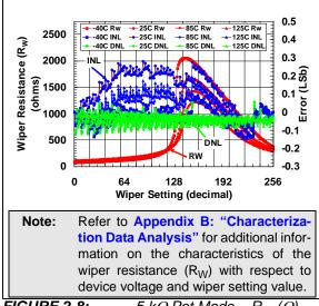
**FIGURE 2-8:** 5 k $\Omega$  Pot Mode –  $R_W(\Omega)$ , INL (LSb), DNL (LSb) vs. Wiper Setting and Ambient Temperature (V<sub>DD</sub> = 1.8V).
