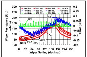
**FIGURE 2-46:** 100 k $\Omega$  Pot Mode –  $R_W(\Omega)$ , INL (LSb), DNL (LSb) vs. Wiper Setting and Ambient Temperature ( $V_{DD} = 3.0V$ ).
