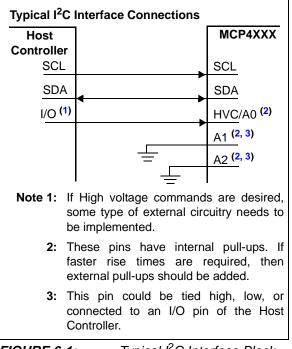
FIGURE 6-1: Typical I<sup>2</sup>C Interface Block Diagram.
