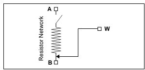
FIGURE 5-2: Resistor Network Shutdown Configuration.
