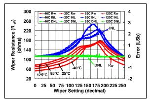
**FIGURE 2-23:** 10 k $\Omega$  Rheo Mode –  $R_W(\Omega)$ , INL (LSb), DNL (LSb) vs. Wiper Setting and Ambient Temperature ( $V_{DD} = 3.0V$ ).
