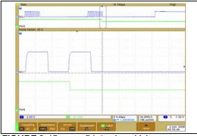
**FIGURE 2-15:**  $5 k\Omega$  – Low-Voltage Decrement Wiper Settling Time (V<sub>DD</sub> = 2.7V) (1 µs/Div).
