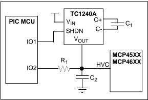
**FIGURE 8-1:** Using the TC1240A to Generate the V<sub>IHH</sub> Voltage.
