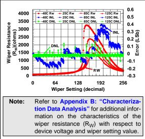
**FIGURE 2-21:** 10 k $\Omega$  Pot Mode –  $R_W(\Omega)$ , INL (LSb), DNL (LSb) vs. Wiper Setting and Ambient Temperature (V<sub>DD</sub> = 1.8V).
