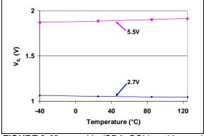
**FIGURE 2-62:** V<sub>IL</sub> (SDA, SCL) vs. V<sub>DD</sub> and Temperature.
