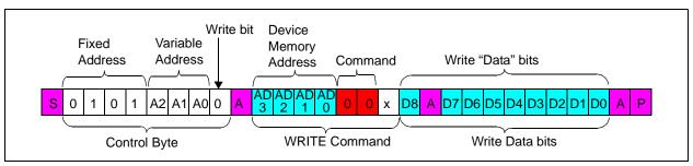
FIGURE 7-2: I<sup>2</sup>C Write Sequence.
