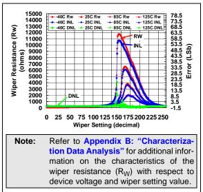
**FIGURE 2-37:** 50 k $\Omega$  Rheo Mode –  $R_W(\Omega)$ , INL (LSb), DNL (LSb) vs. Wiper Setting and Ambient Temperature (V<sub>DD</sub> = 1.8V).
