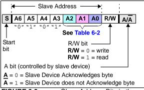
**FIGURE 6-9:** Slave Address Bits in the  $l^2C$  Control Byte.
