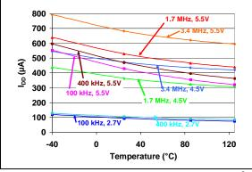
**FIGURE 2-1:** Device Current ( $I_{DD}$ ) vs.  $f^2C$ Frequency ( $f_{SCL}$ ) and Ambient Temperature ( $V_{DD} = 2.7V$  and 5.5V).
