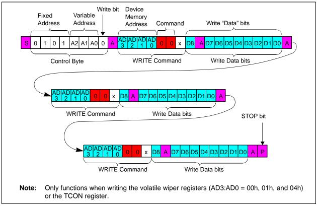
FIGURE 7-3: I<sup>2</sup>C Continuous Volatile Wiper Write.
