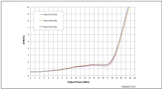
FIGURE 5-3: DYNAMIC EVM VERSUS OUTPUT POWER, WITH MSCS7-40 MHz
