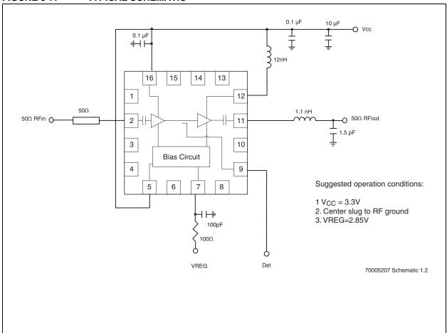
$0.1~\mu F$ O Vcc 1 µF Ţ ٠Ĥ٢ 3 12nH 16 15 14 13 1 12 50Ω 2.0 nH 50Ω RFin O -O <sup>50Ω RFout</sup> 11 2.0 pF 3.0 pF 3 10 Bias Circuit 4 9 Suggested operation conditions: 5 8 6 7 1 Vcc = 3.3 V2. Center slug to RF ground <del>|</del> | | | | | | | 3. VREG=2.85V 100pF Ω0 Det VREG 70005207 Schematic 2.1
