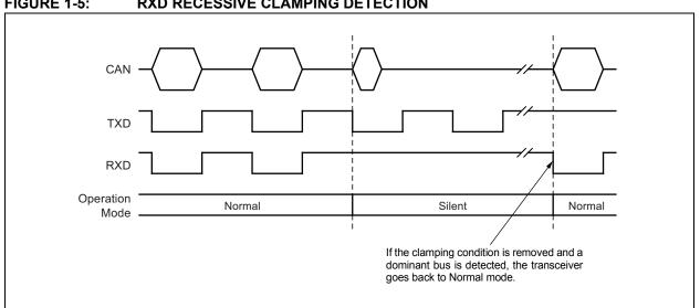
FIGURE 1-5: **RXD RECESSIVE CLAMPING DETECTION**
