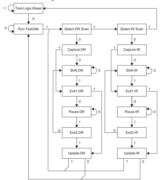
Figure 24-2. TAP Controller State Diagram
