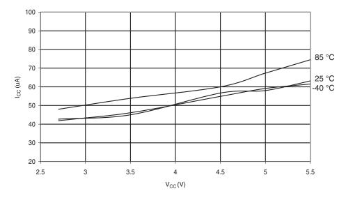
Figure 29-51. Programming Current vs.  $V_{\rm CC}$
