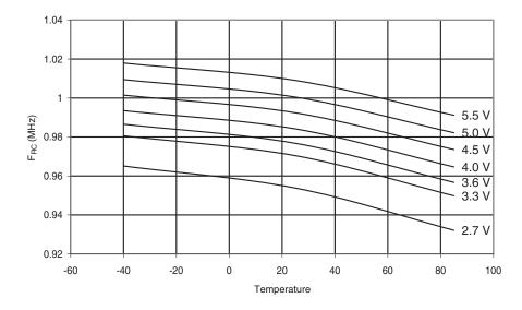
Figure 29-45. Calibrated 1MHz RC Oscillator Frequency vs.  $V_{\rm CC}$
