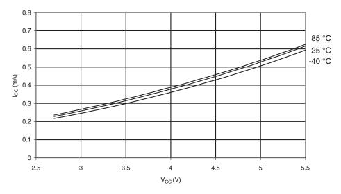
Figure 29-12. Idle Supply Current vs.  $V_{CC}$  (External Oscillator, 32kHz)
