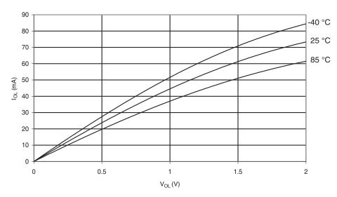
Figure 29-24. I/O Pin Sink Current vs. Output Voltage (V<sub>CC</sub> = 3V)
