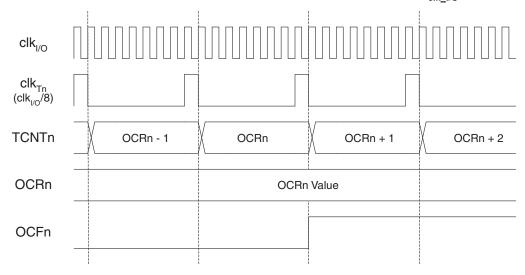
Figure 18-11 shows the setting of OCF2 and the clearing of TCNT2 in CTC mode.
