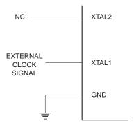
When this clock source is selected, start-up times are determined by the SUT fuses as shown in Table 9-10.
