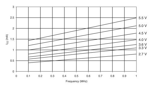
Figure 29-53. Reset Supply Current vs. Frequency
