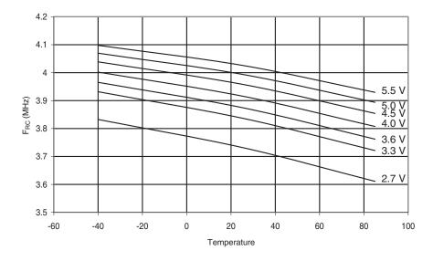
Figure 29-39. Calibrated 4MHz RC Oscillator Frequency vs.  $V_{\rm CC}$
