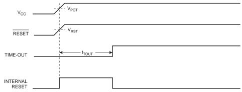
Figure 11-3. MCU Start-up, RESET Extended Externally
