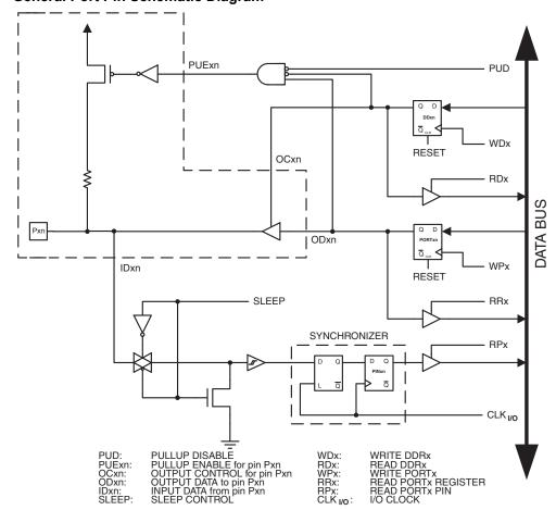
Figure 25-4. General Port Pin Schematic Diagram<sup>(1)</sup>
