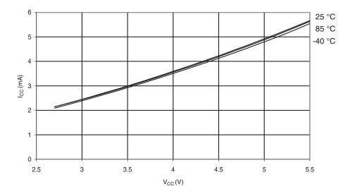
Figure 29-5. Active Supply Current vs.  $V_{CC}$  (Internal RC Oscillator, 1MHz)
