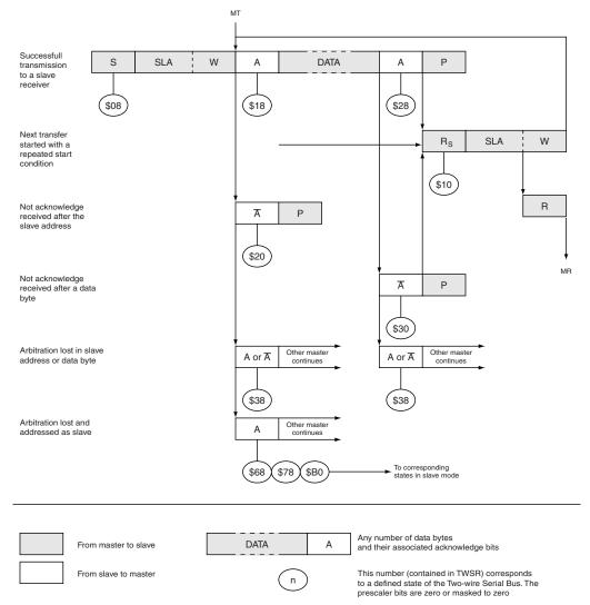
Figure 21-12. Formats and States in the Master Transmitter Mode
