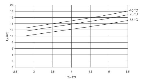
Figure 29-48. ADC Current vs.  $V_{CC}$  (AREF = AVCC)
