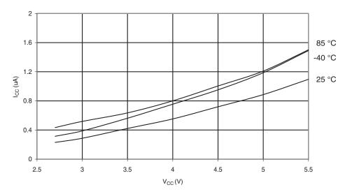
Figure 29-14. Power-down Supply Current vs. V<sub>CC</sub> (Watchdog Timer Enabled)
