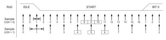
When the clock recovery logic detects a high (idle) to low (start) transition on the RxD line, the start bit detection sequence is initiated. Let sample 1 denote the first zero-sample as shown in the figure. The clock recovery logic then uses samples 8, 9, and 10 for Normal mode, and samples 4, 5, and 6 for Double Speed mode (indicated with sample numbers inside boxes on the figure), to decide if a valid start bit is received. If two or more of these three
