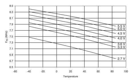
Figure 29-36. Calibrated 8MHz RC Oscillator Frequency vs.  $V_{\text{CC}}$
