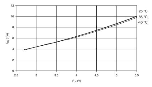
Figure 29-4. Active Supply Current vs. V<sub>CC</sub> (Internal RC Oscillator, 4MHz)
