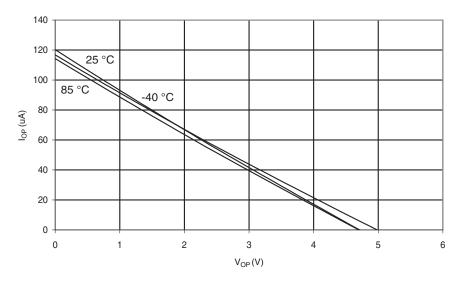
Figure 29-18. I/O Pin Pull-up Resistor Current vs. Input Voltage (V<sub>CC</sub> = 2.7V)
