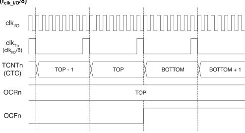
Figure 18-11. Timer/Counter Timing Diagram, Clear Timer on Compare Match Mode, with Prescaler (f<sub>clk I/O</sub>/8)
