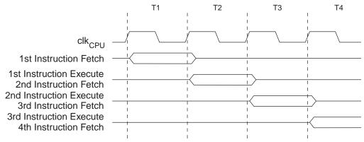
Figure 7-5 shows the internal timing concept for the Register File. In a single clock cycle an ALU operation using two register operands is executed, and the result is stored back to the destination register.
