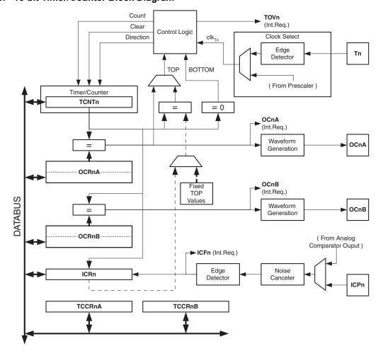
Figure 17-1. 16-bit Timer/Counter Block Diagram<sup>(1)</sup>
