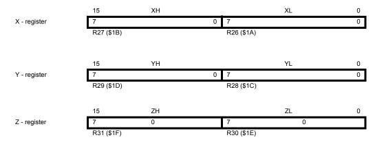
In the different addressing modes these address registers have functions as fixed displacement, automatic increment, and automatic decrement (see the AVR Instruction Set Manual on www.microchip.com for details).
