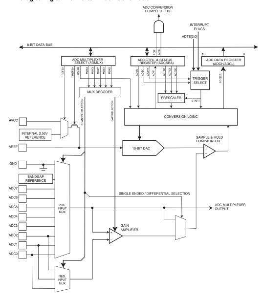
Figure 23-1. Analog to Digital Converter Block Schematic
