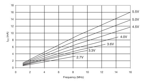
Figure 29-3. Active Supply Current vs. V<sub>CC</sub> (Internal RC Oscillator, 8MHz)
