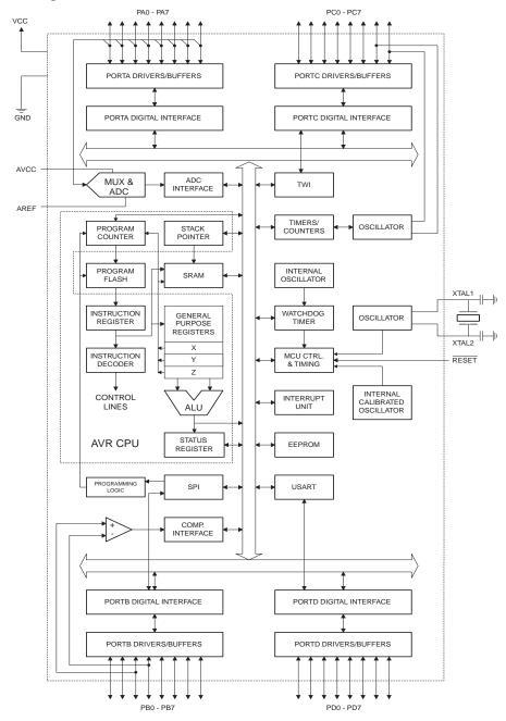
The AVR® core combines a rich instruction set with 32 general purpose working registers. All the 32 registers are directly connected to the Arithmetic Logic Unit (ALU), allowing two independent registers to be accessed in one
