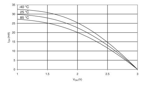
Figure 29-23. I/O Pin Sink Current vs. Output Voltage (V<sub>CC</sub> = 5V)
