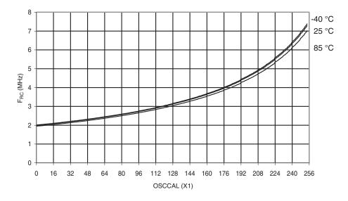
Figure 29-41. Calibrated 2MHz RC Oscillator Frequency vs. Temperature
