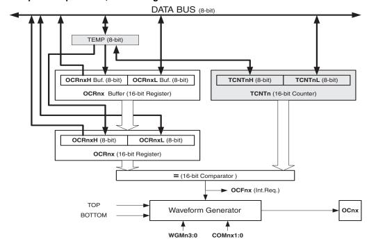
Figure 17-4. Output Compare Unit, Block Diagram
