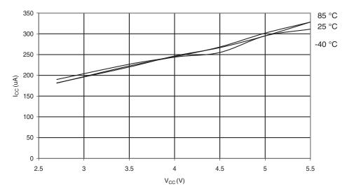
Figure 29-49. AREF External Reference Current vs.  $V_{\rm CC}$
