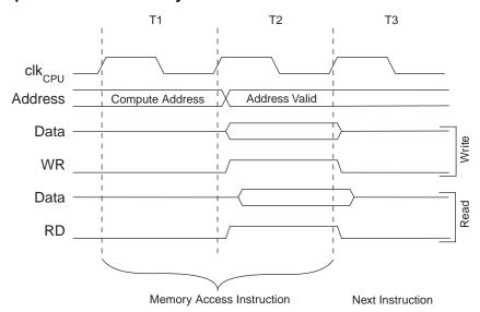
Figure 8-3. On-chip Data SRAM Access Cycles
