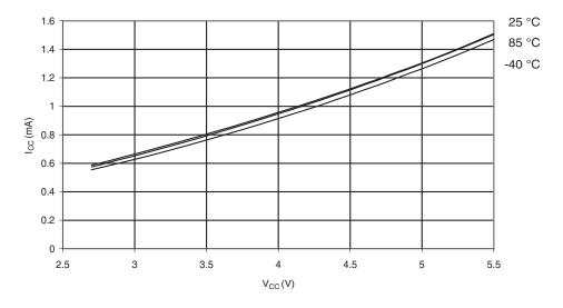
Figure 29-6. Active Supply Current vs. V<sub>CC</sub> (External Oscillator, 32kHz)
