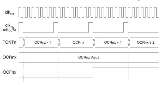
Figure 17-12 shows the count sequence close to TOP in various modes. When using phase and frequency correct PWM mode the OCR1x Register is updated at BOTTOM. The timing diagrams will be the same, but TOP should be replaced by BOTTOM, TOP-1 by BOTTOM+1 and so on. The same renaming applies for modes that set the TOV1 Flag at BOTTOM.
