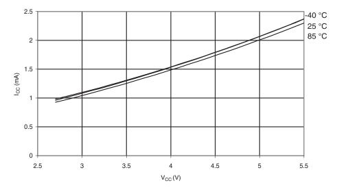
Figure 29-11. Idle Supply Current vs.  $V_{CC}$  (Internal RC Oscillator, 1MHz)
