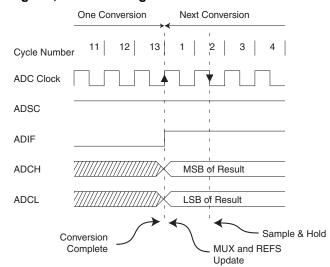
Figure 23-7. ADC Timing Diagram, Free Running Conversion
