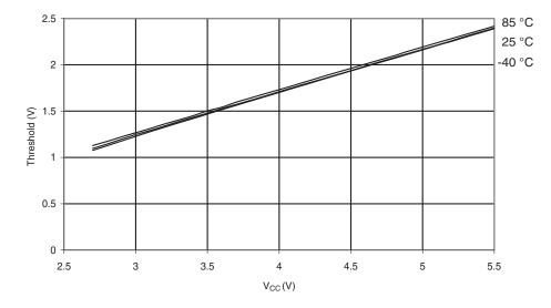
Figure 29-27. I/O Pin Input Hysteresis vs.  $V_{\text{CC}}$
