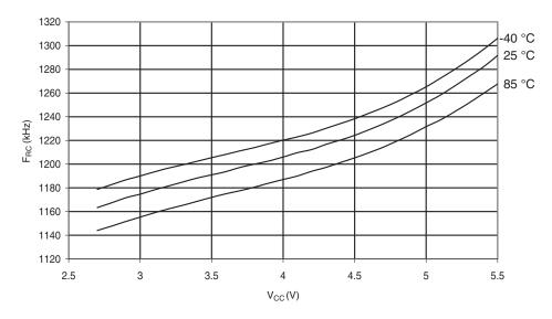
Figure 29-35. Calibrated 8MHz RC Oscillator Frequency vs. Temperature
