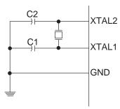
The Oscillator can operate in three different modes, each optimized for a specific frequency range. The operating mode is selected by the fuses CKSEL3:1 as shown in Table 9-3.
