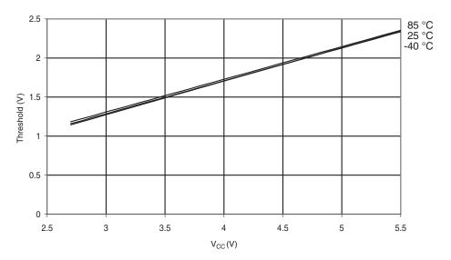
Figure 29-30. Reset Input Pin Hysteresis vs.  $V_{\rm CC}$
