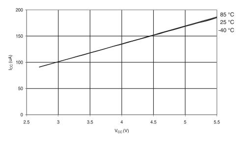
Figure 29-50. Analog Comparator Current vs. V<sub>CC</sub>
