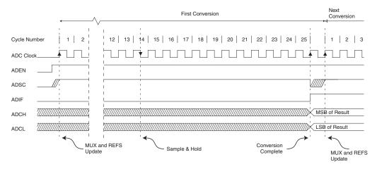
Figure 23-5. ADC Timing Diagram, Single Conversion
