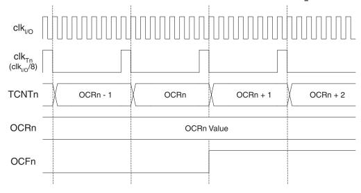
Figure 15-11 shows the setting of OCF0 and the clearing of TCNT0 in CTC mode.
