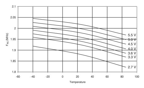
Figure 29-42. Calibrated 2MHz RC Oscillator Frequency vs. V<sub>CC</sub>
