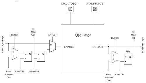
Table 25-3 summaries the scan registers for the external clock pin XTAL1, Oscillators with XTAL1/XTAL2 connections as well as 32kHz Timer Oscillator.
