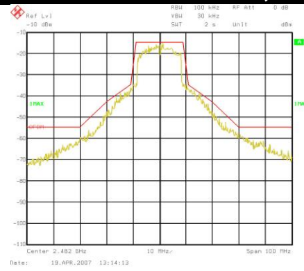
Typical OFDM Output Spectrum at +29dBm, 2.482GHz ( V_c = V_{cc} = 5.0V , V_{ref} = 2.9V , I_{cq} = 120mA , 64QAM/54Mbps)
