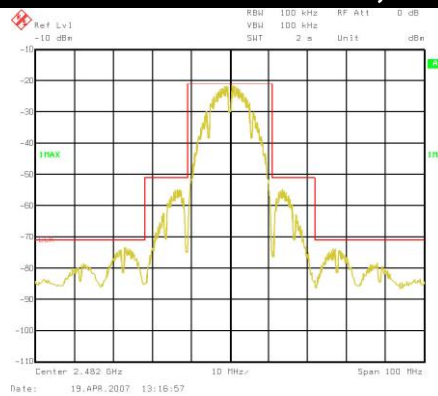
Typical 1Mbps DSSS output spectrum at +28dBm, 2.482GHz ( V_c = V_{cc} = 5.0V , V_{ref} = 2.9V , I_{cq} = 120mA , 1Mbps DSSS)
