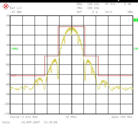
Typical 1Mbps DSSS output spectrum at +28dBm, 2.412GHz ( V_c = V_{cc} = 5.0V , V_{ref} = 2.9V , I_{cq} = 120mA , 1Mbps DSSS)
