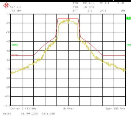
Typical OFDM Output Spectrum at +29dBm, 2.412GHz ( V_c = V_{cc} = 5.0V , v_{ref} = 2.9V , I_{cq} = 120mA , 64QAM/54Mbps)
