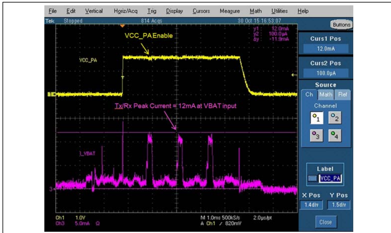
FIGURE 3-1: AVERAGE CURRENT CONSUMPTION DURING ADVERTISING
