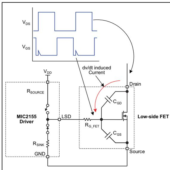
**FIGURE 4-10:** *dv/dt-Induced Turn-on.*
