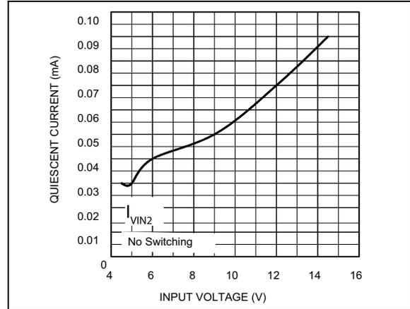
**FIGURE 2-4:** Quiescent Current 2 vs. Input Voltage.
