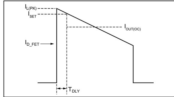
**FIGURE 4-15:** Overcurrent Waveform.
