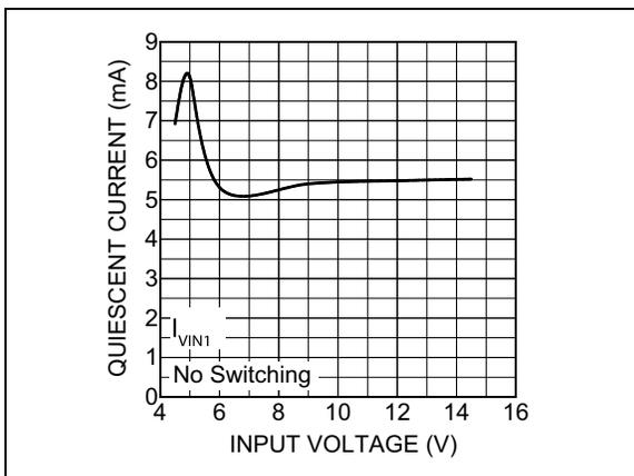
**FIGURE 2-3:** Quiescent Current 1 vs. Input Voltage.
