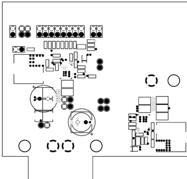
Figure 14. MIC24056 Evaluation Board Mid-Layer 1 (Ground Plane)
