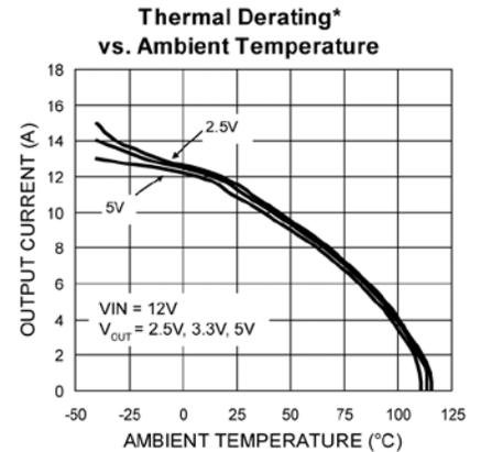
**Die Temperature\*** : The temperature measurement was taken at the hottest point on the MIC24056 case mounted on a 5 square inch 4 layer, 0.62 inch, FR-4 PCB with 2oz finish copper weight per layer; see Thermal Measurement section. Actual results will depend upon the size of the PCB, ambient temperature and proximity to other heat emitting components.
