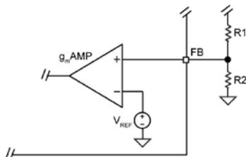
**Figure 9. Voltage-Divider Configuration**
