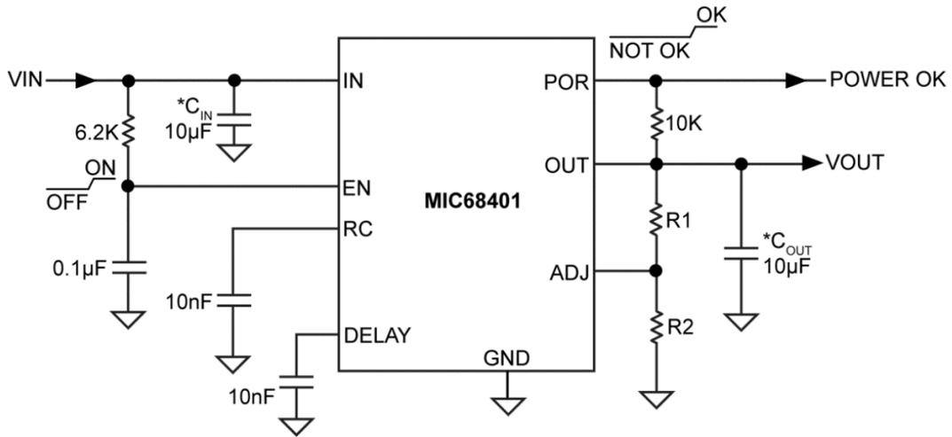
\*MINIMUM CAPACITANCE. FOR GUIDANCE ON THE VALUE OF C<sub>IN</sub> AND C<sub>OUT</sub>, PLEASE REFER TO THE APPLICATIONS INFORMATION SECTION
