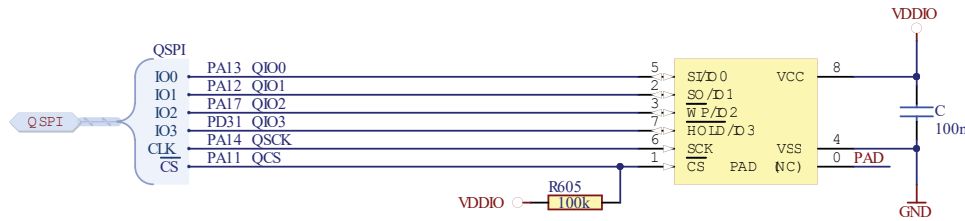
Figure 59-6. Schematic Example with QSPI Data Flash
