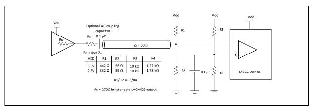
Figure 7. Input driven by a single ended output
