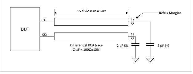
Figure 19. Test Circuit
