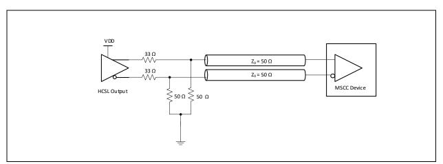
Figure 3. Input driven by source terminated HCSL
