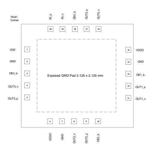
Figure 2. Pin Diagram
