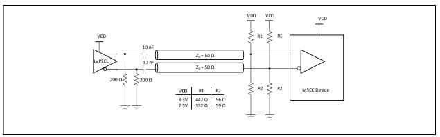
Figure 5. Input driven by AC coupled LVPECL output
