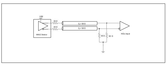
Figure 9. Receiver terminated HCSL
