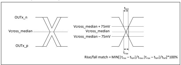
Figure 16. Single-Ended Measurement Points for Rise and Fall Time Matching
