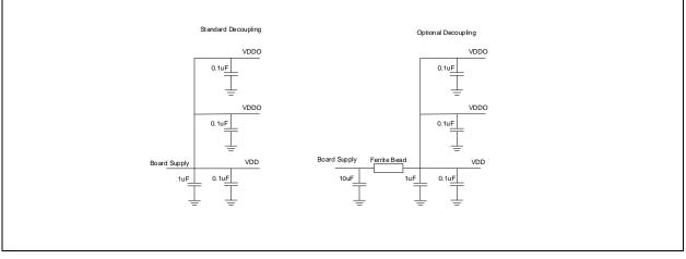
Figure 10. Power Supply Filtering
