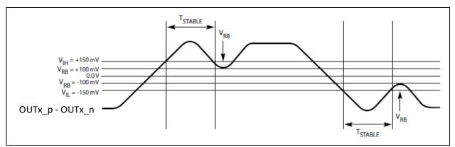
Figure 18. Differential Measurement Points for Ringback
