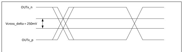
Figure 15. Single-Ended Measurement Points for Delta Cross Point
