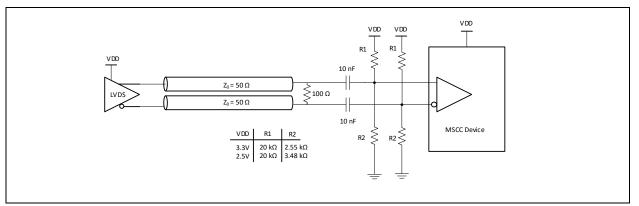
Figure 6. Input driven by AC coupled LVDS
