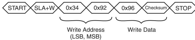
Figure 6-2. Example of a Write To Address 0x1234 With a Checksum
