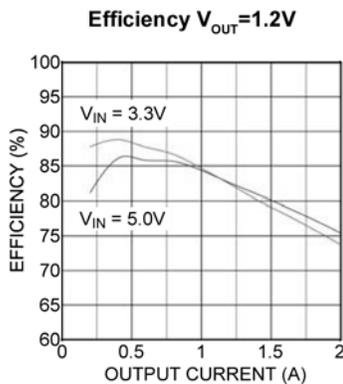
**Figure 2. Efficiency Curve**
