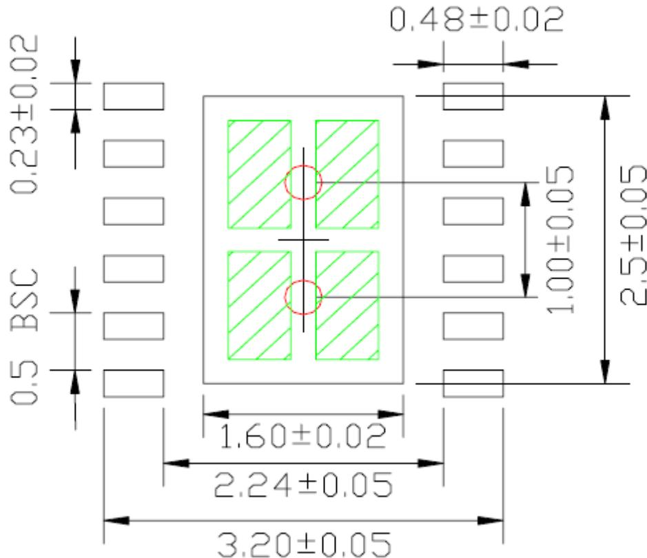
**Red circle** indicates Thermal Via. Size should be 300-350  $\mu\text{m}$  in diameter, 1.00 mm pitch and should be connected to GND plane for maximum thermal performance.
