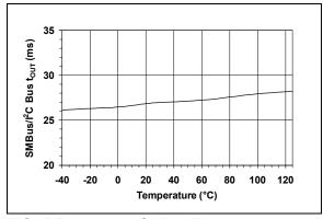
FIGURE 2-16: SMBus Time-out vs. Temperature
