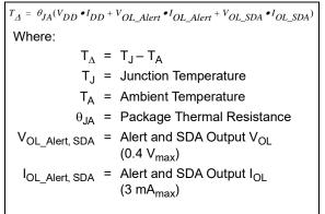
At room temperature ( $T_A = +25^{\circ}C$ ) with maximum  $I_{DD} = 500 \ \mu A$  and  $V_{DD} = 3.6V$ , the self-heating due to power dissipation  $T_{\Delta}$  is +0.2°C for the DFN-8 package and +0.5°C for the TSSOP-8 package.
