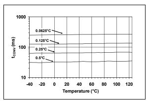
FIGURE 2-12: Temperature Conversion Time vs. Temperature
