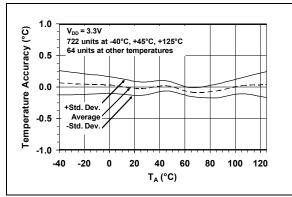
FIGURE 2-1: Temperature Accuracy
