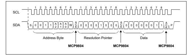
**FIGURE 5-8:** Timing Diagram for Changing T<sub>A</sub> Resolution to +0.0625°C < 0000 0011>b (see Section 4.0 "Serial Communication")
