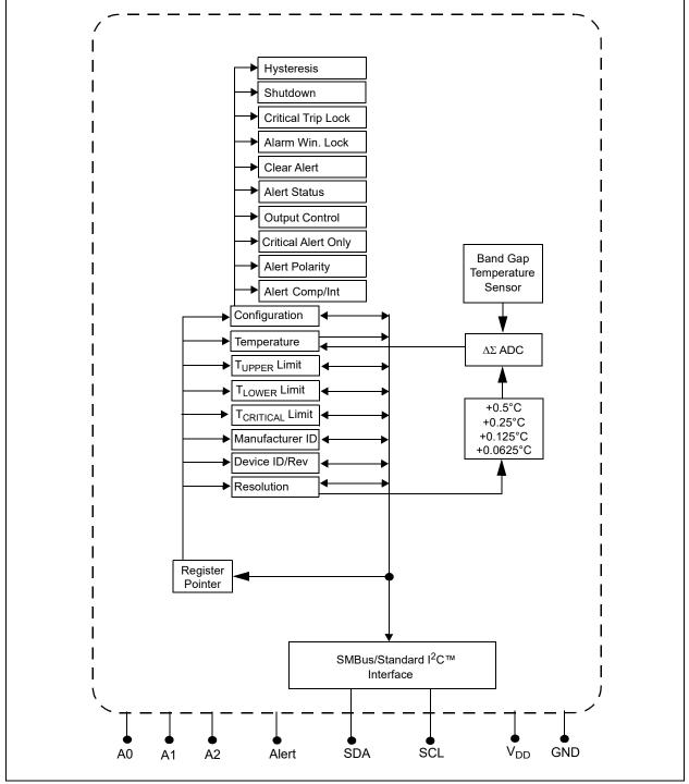
FIGURE 5-1: Functional Block Diagram
