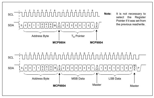
**FIGURE 5-5:** Timing Diagram for Reading +25.25°C Temperature from the T<sub>A</sub> Register (see **Section 4.0 "Serial Communication**")
