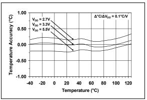
FIGURE 2-10: Temperature Accuracy vs. Supply Voltage
