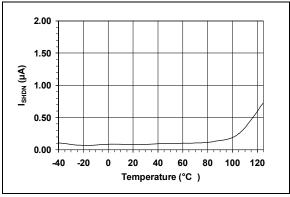
FIGURE 2-8: Shutdown Current vs. Temperature
