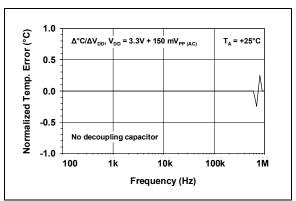
FIGURE 2-11: Power Supply Rejection vs. Frequency
