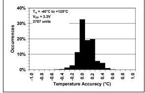
**FIGURE 2-2:** Temperature Accuracy Histogram,  $T_A = -40$ °C to +125°C
