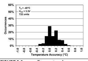
**FIGURE 2-6:** Temperature Accuracy Histogram,  $T_A = -40$  °C
