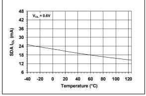
FIGURE 2-14: SDA I<sub>OL</sub> vs. Temperature
