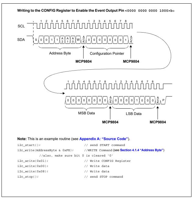
FIGURE 5-2: Timing Diagram for Writing to the Configuration Register (see Section 4.0 "Serial Communication")
