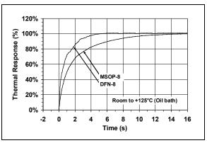
FIGURE 2-15: Package Thermal Response
