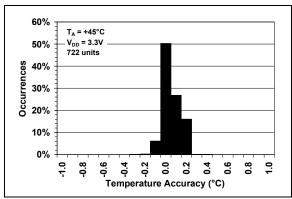
**FIGURE 2-4:** Temperature Accuracy Histogram,  $T_A = +45$ °C
