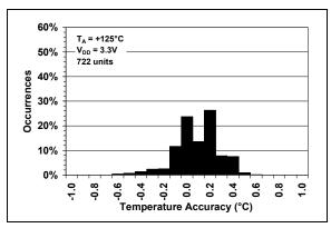
**FIGURE 2-5:** Temperature Accuracy Histogram,  $T_A = +125$ °C
