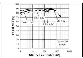
FIGURE 2-4: Efficiency ( $V_{OUT} = 1.5V$ ) vs. Output Current.
