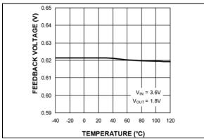
FIGURE 2-14: Feedback Voltage vs. Temperature.
