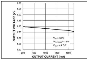
FIGURE 2-11: Load Regulation (CCM).
