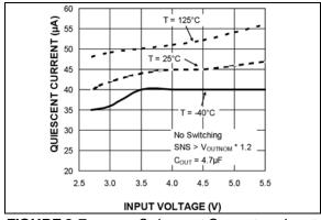
FIGURE 2-7: Quiescent Current vs. Input Voltage.
