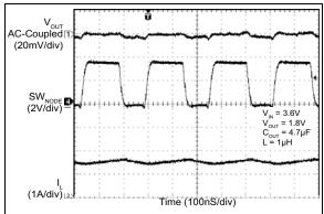
FIGURE 2-19: Switching Waveform Continuous Mode (1.5A).
