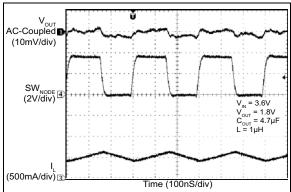
FIGURE 2-18: Switching Waveform Continuous Mode (500 mA).
