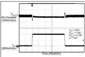
FIGURE 2-21: Load Transient (50 mA to 1A).
