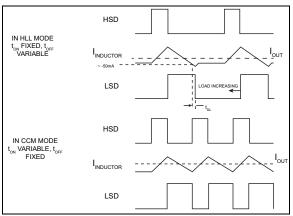
**FIGURE 5-1:** Transition Between CCM Mode and HLL Mode.
