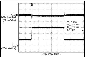
FIGURE 2-22: Load Transient (200 mA to 600 mA).
