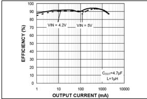
**FIGURE 2-1:** Efficiency  $(V_{OUT} = 3.3V)$  vs. Output Current.
