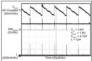
FIGURE 2-16: Switching Waveform Discontinuous Mode (1 mA).
