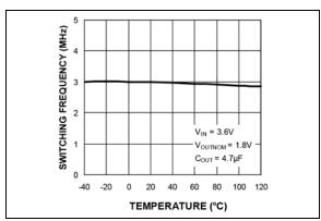
**FIGURE 2-15:** Switching Frequency vs. Temperature.
