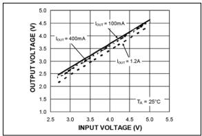
**FIGURE 2-13:** Maximum Output Voltage vs. Input Voltage.
