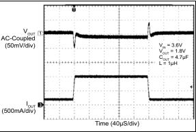
FIGURE 2-23: Load Transient (200 mA to 1A).
