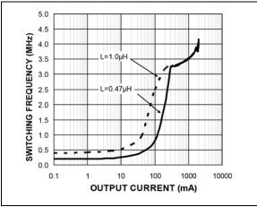
**FIGURE 5-3:** Switching Frequency vs. Output Current.
