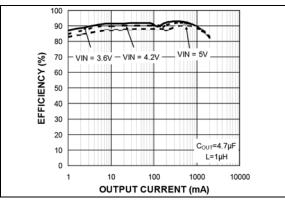
**FIGURE 2-2:** Efficiency  $(V_{OUT} = 2.5V)$  vs. Output Current.
