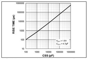
**FIGURE 2-5:**  $V_{OUT}$  Rise Time vs.  $C_{SS}$ .
