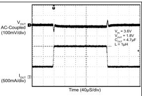
**FIGURE 2-24:** Load Transient (200 mA to 1.5A).
