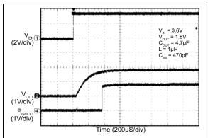
FIGURE 2-28: Power Good During Startup.
