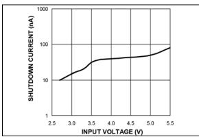
FIGURE 2-8: Shutdown Current vs. Input Voltage.
