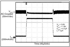
FIGURE 2-20: Load Transient (50 mA to 750 mA).
