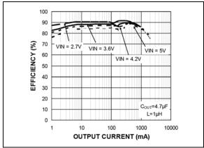
FIGURE 5-2: Efficiency Under Load.
