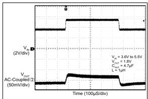
**FIGURE 2-25:** Line Transient (3.6V to 5.5V at 1.5A).
