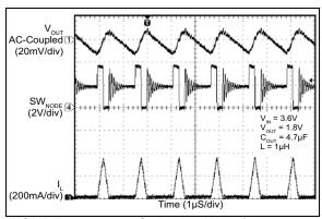
FIGURE 2-17: Switching Waveform Discontinuous Mode (50 mA).
