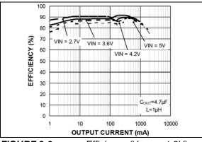
**FIGURE 2-3:** Efficiency  $(V_{OUT} = 1.8V)$  vs. Output Current.
