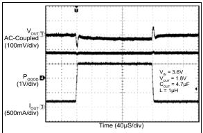
FIGURE 2-26: Power Good Load Transient (200 mA to 1.5A).
