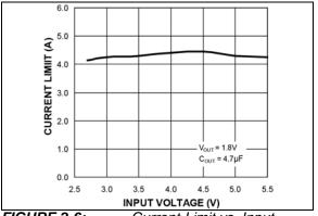
FIGURE 2-6: Current-Limit vs. Input Voltage.
