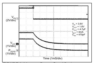
FIGURE 2-29: Power Good During Shutdown (MIC23159).
