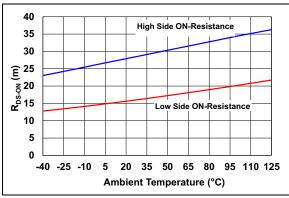
FIGURE 2-4: R<sub>DS-ON</sub> vs. Temperature.
