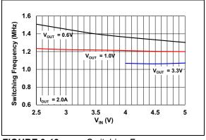
**FIGURE 2-12:** Switching Frequency vs. Input Voltage.
