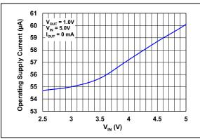
FIGURE 2-1: Operating Supply Current vs. Input Voltage, Switching.
