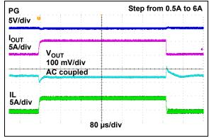
FIGURE 2-23: Load Transient Response.
