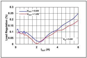
**FIGURE 2-10:** Load Regulation: V<sub>OUT</sub> Voltage Variation vs. I<sub>OUT</sub>.
