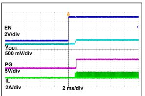
EN Turn-On into Pre-Biased **FIGURE 2-17:** Output ( $V_{pre-bias} = 0.8V$ ).
