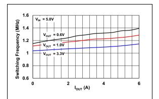
FIGURE 2-11: Switching Frequency vs. Output Current.
