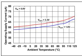
FIGURE 2-3: Operating Supply Current vs. Temperature, Switching.
