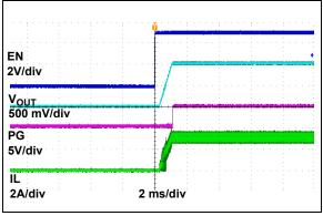
FIGURE 2-15: EN Turn-On,  $R_{LOAD} = 0.3 \Omega$ .
