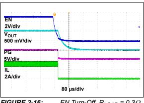
$\overline{EN \ Turn-Off}, \ R_{LOAD} = 0.3 \Omega.$ FIGURE 2-16:
