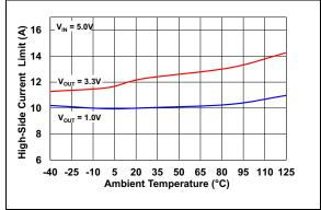
**FIGURE 2-2:** High-Side Current Limit vs. Temperature (closed-loop).
