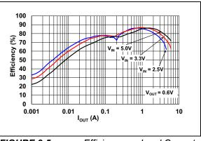
FIGURE 2-5: Efficiency vs. Load Current.
